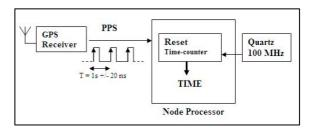
Figure 9: Embedded GPS synchronization principle.
