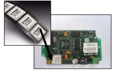
Figure 8: GPS receiver on the mother board.
