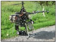
Figure 12: LCPC U.A.V. for structure inspection
