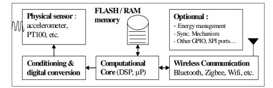
Figure 1: Typical wireless sensor functional layouts.
