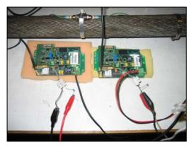
Figure 10: Synchronization test-bench for two wireless sensors.
