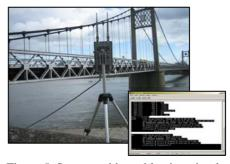
Figure 5: Sensors addressable via a simple Wi-Fi Access Point and the Telnet service.
