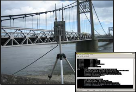
Figure 5: Sensors addressable via a simple Wi-Fi Access Point and the Telnet service.
