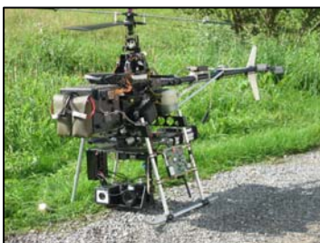
Figure 12: LCPC U.A.V. for structure inspection
