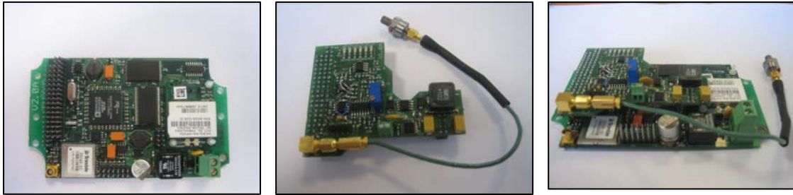
Figure 2: mother board, daughter board, and the both plugged one to the other.
