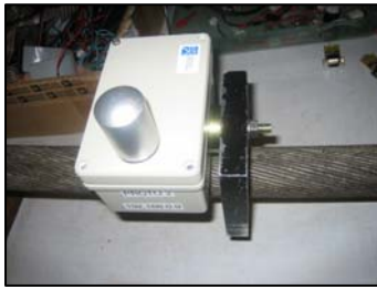
Figure 14: LCPC wireless sensor for cable monitoring.
