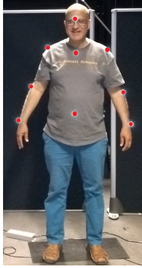
Fig. 3. Motion capture markers position
