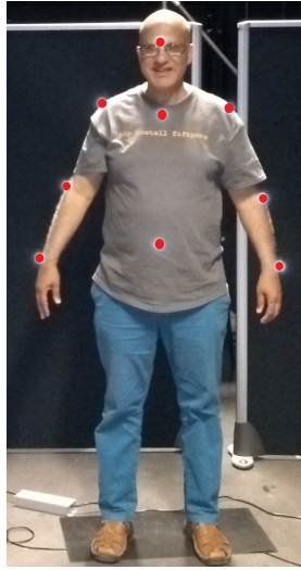
Fig. 3. Motion capture markers position
