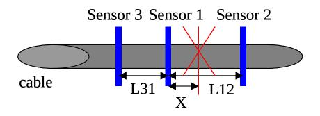
Figure 2. Rupture localization by acoustic sensors
