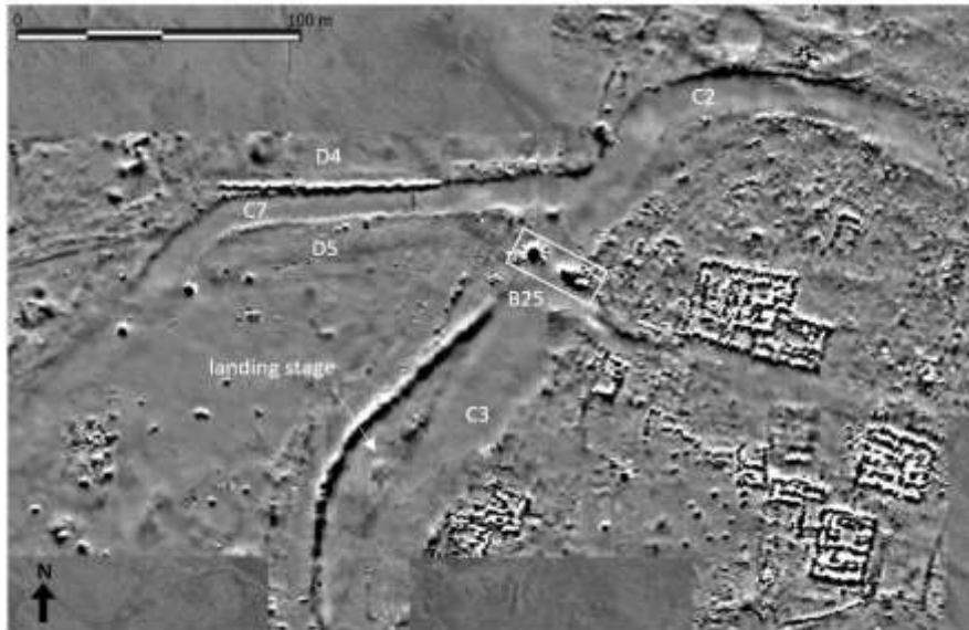
Fig. 5. Geomagnetic image showing the hydraulic network of the north of Larsa. White box highlights the magnetic anomalies of the baked bricks piers of the bridge B25 (north). © L. Darras and Mission of Larsa-Uwaili, 2022.
