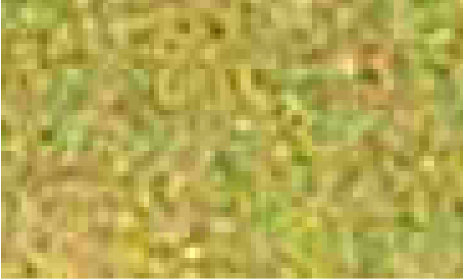
Figure 9: Noisy pattern of a flat zone in an image compressed by JPEG. Pixels of the same colors are usually in small groups rather than appearing individually due to the interpolation of demosaicing, and the pixels in a 8 \times 8 block are similar due to the JPEG compression processed on 8 \times 8 blocks.
