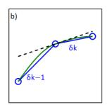
Figure 4: Slopes for PCHIP.  $\delta_k$  and  $\delta_{k-1}$  are the two slopes of the piecewise linear interpolant on either side of the breakpoint
