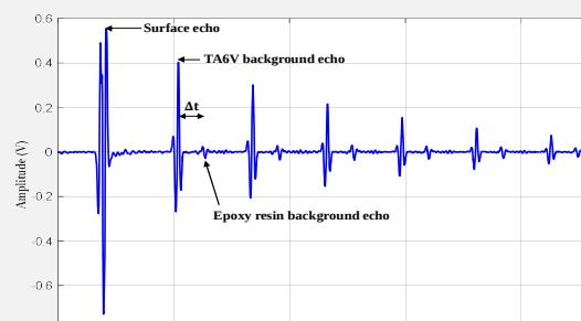
$$e_{Epoxy} = \frac{c_{L-Epoxy} \times \Delta t_{corr}}{2} \cong 0.1357 \text{ mm}$$
