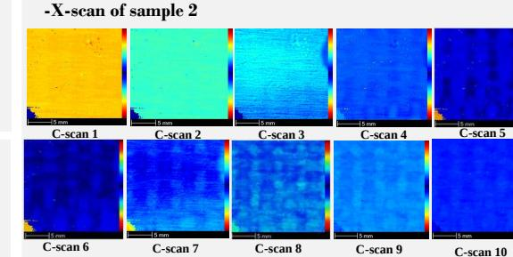
Size of the X-scan gate = 20 ns  $\Rightarrow d(\text{Epoxy})=23 \mu\text{m}$ ,  $d(\text{Composite}) = 29.2 \mu\text{m}$
