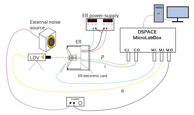
Fig. 16 Sketch of the entire experimental setup.
