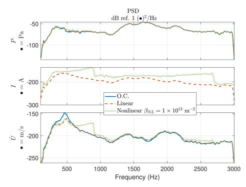
Fig. 24 Auto-PSDs of pressure, electrical current and velocity between 100 and 3000 Hz, in case of open circuit (O.C.) loudspeaker (solid blue), Linear with  $\mu_M \ \mu_K \ 1$  and  $R_{at} \ \rho_0 c_0$  (dashed red) and Duffing with  $\beta_{NL} \ 1 \times 10^{13}$  m<sup>-2</sup> (dotted green) target dynamics.
