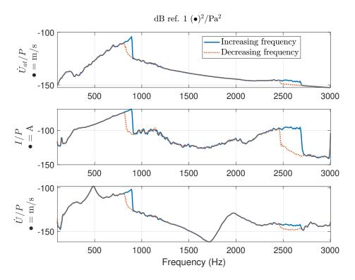
Fig. 28 PSDs of target velocity, electrical current and actual velocity, divided by the PSD of pressure, for *forward* or *backard* linear variation of frequency in the chirp excitation. The terms of the target dynamics are fixed as  $\mu_M \ \mu_K \ 1$ ,  $R_{at} \ \rho_0 c_0$  and  $\beta_{NL} \ 1 \times 10^{13} \ m^{-2}$ .
