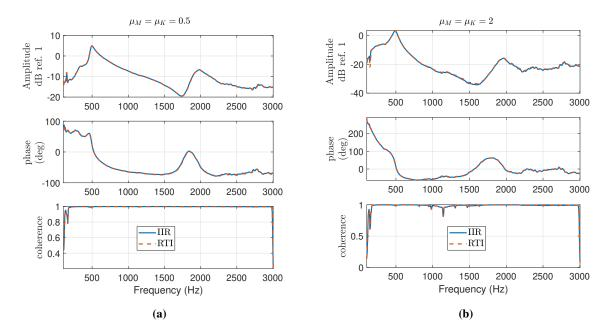
Fig. 29 Mobility obtained by targeting a linear SDOF dynamics of the ER with  $\mu_M \ \mu_K \ 0.5$  (a) and  $\mu_M \ \mu_K \ 2$  (a), and  $R_{at} \ \rho_0 c_0$ , by either the IIR (solid blue line) or the RTI (dashed red line).
