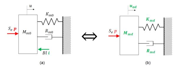
Fig. 4 Sketches of the SDOF model of the ER (a) and of the target SDOF LTI resonator (b).
