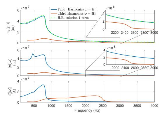
Fig. 10 Fundamental and third Harmonics of the desired displacement amplitude  $|u_d j\omega|$ , and actual displacement amplitude  $|u j\omega|$ , in case of Duffing desired dynamics of the ER (with  $\mu_M \ \mu_K \ 1$ ,  $R_{at} \ \rho_0 c_0$  and  $\beta_{NL} \ 1 \times 10^{13} \ m^{-2}$ ). The target displacement fundamental harmonics are compared to the Harmonic-Balance 1-term analytical solution. The zoom of  $|u_d j\omega|$  and  $|u j\omega|$  is around the secondary jump.
