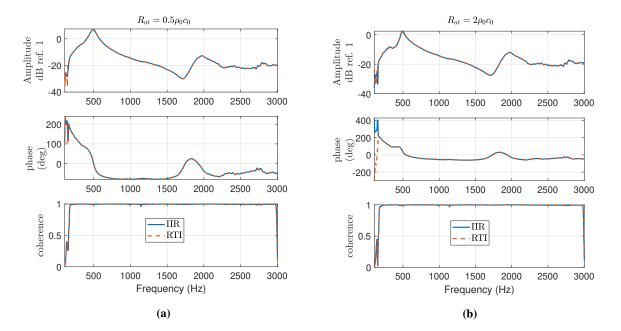
**Fig. 32** Mobility obtained by targeting a linear SDOF dynamics of the ER with  $R_{at}$   $0.5\rho_0c_0$  (a) and  $R_{at}$   $2\rho_0c_0$  (a), and  $\mu_M$   $\mu_K$  1, by either the IIR (solid blue line) or the RTI (dashed red line).
