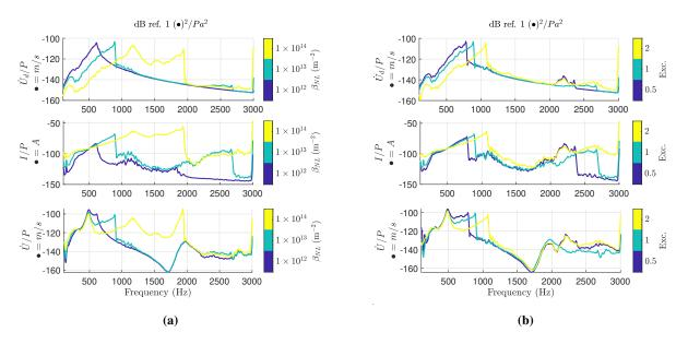
Fig. 26 Auto-PSDs of target velocity, electrical current and actual velocity, divided by the auto-PSD of pressure, for varying  $\beta_{NL}$  (a) and excitation amplitude (b).
