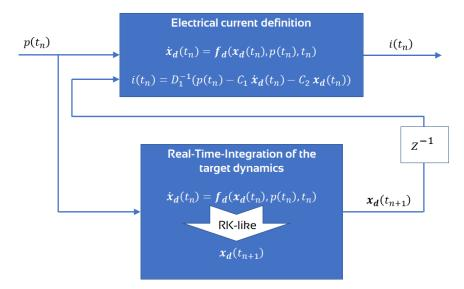
Fig. 1 Block diagram of the two-steps control algorithm.
