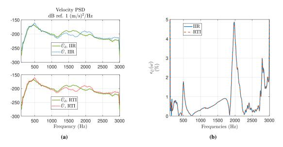
Fig. 19 Auto-PSDs of desired  $U_d$  and actual U velocity (a), and corresponding error percentage (b), obtained by targeting a linear SDOF dynamics of the ER with  $\mu_M \ \mu_K \ 1$  and  $R_{at} \ \rho_0 c_0$  by either the IIR or the RTI.
