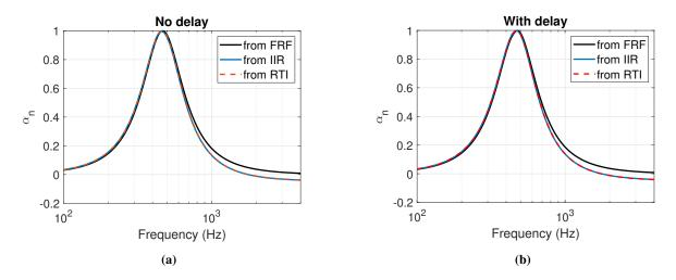
Fig. 6 Simulated normal absorption coefficients obtained directly in frequency domain from  $H_j\omega$  (in black) compared with the values obtained by the IIR (in blue) and RTI (in dashed red) time implementations of the controller. In (a) no time delay is assumed, while in (b) a time delay of  $2 \times 10^{-5}$  seconds is considered. The target impedance operator is set with values:  $\mu_M \ \mu_K \ 1$  and  $R_{at} \ \rho_0 c_0$ .
