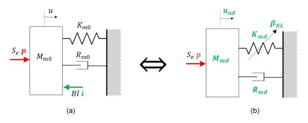
Fig. 7 Sketches of the SDOF model of the ER (on the left) and of the target SDOF Duffing resonator (on the right).
