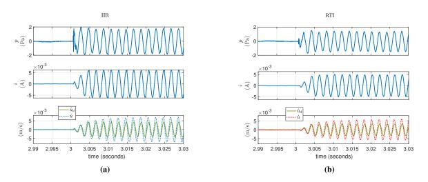
Fig. 17 Time histories of pressure pt, electrical current *it* and desired and measured velocities ( $u_d$  and ut respectively) on the speaker diaphragm, when an external sound source emitting a pure sine at 500 Hz, is activated after t 3 seconds. A linear SDOF dynamics of the ER with  $\mu_M \ \mu_K \ 1$  and  $R_{at} \ \rho_0 c_0$  is targeted either by the IIR (a) or by the RTI (b) implementation strategy.
