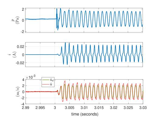
Fig. 21 Time histories of pressure *pt*, electrical current *it*, target and measured velocities ( $u_d$  and *ut* respectively) on the speaker diaphragm. An external sound source emitting a pure sine at 700 Hz, is activated after *t* 3 seconds. The linear target SDOF dynamics of the ER has  $\mu_M \ \mu_K \ 1$ ,  $R_{at} \ \rho_0 c_0$  and  $\beta_{NL} \ 1 \times 10^{13} \text{ m}^{-2}$ .
