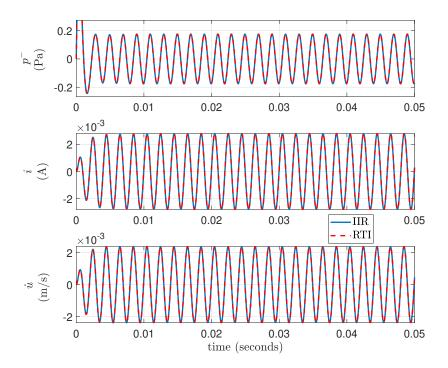
Fig. 5 Simulated time histories of ER velocity ut, reflected pressure  $p^-t$  and electrical current signals it, for harmonic normally-incident pressure wave pt of amplitude 1 Pa at 500 Hz, in case of IIR (in solid blue) and RTI (in dashed red) controller implementations.
