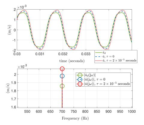
Fig. 9 Time history zoom in the stationary regime (top) and DFTs amplitudes zoom at the fundamental harmonic 700 Hz (bottom), of target  $u_d$  and actual u velocities, in case of Duffing desired dynamics of the ER. Both synchronous ( $\tau$  0) and delayed ( $\tau$  2 × 10<sup>-5</sup> seconds) simulation results, are showed.
