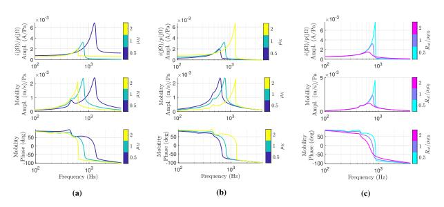
Fig. 12 Amplitude of the fundamental harmonics of the simulated stationary responses of the ER to harmonic excitation p, in terms of electrical current and acoustic mobility, in case of varying  $\mu_M$  (a),  $\mu_K$  (b) and  $R_{at}$  (c).
