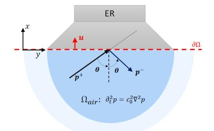
Fig. 2 ER interfacing with a semi-infinite acoustic domain.
