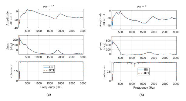
Fig. 30 Mobility obtained by targeting a linear SDOF dynamics of the ER with  $\mu_M$  0.5 (a) and  $\mu_M$  2 (a),  $\mu_K$  1 and  $R_{at}$   $\rho_0 c_0$ , by either the IIR (solid blue line) or the RTI (dashed red line).
