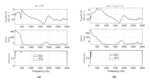
Fig. 31 Mobility obtained by targeting a linear SDOF dynamics of the ER with  $\mu_K 0.5$  (a) and  $\mu_K 2$  (a),  $\mu_M 1$  and  $R_{at} \rho_0 c_0$ , by either the IIR (solid blue line) or the RTI (dashed red line).
