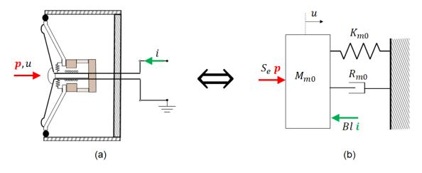
Fig. 3 Sketch of the ER (a) and its SDOF piston-mode model (b) employed in the control synthesis.
