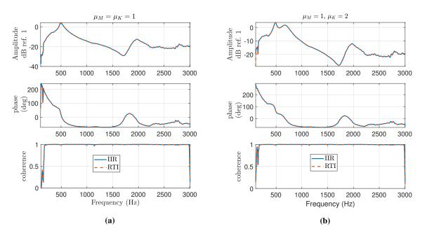
**Fig. 18** Mobility (b) obtained by targeting a linear SDOF dynamics of the ER with  $\mu_M \ \mu_K \ 1$  and  $R_{at} \ \rho_0 c_0$  (a) and  $\mu_M \ 1, \mu_K \ 2$  and  $R_{at} \ \rho_0 c_0$  (b) by either the IIR (solid blue line) or the RTI (dashed red line).
