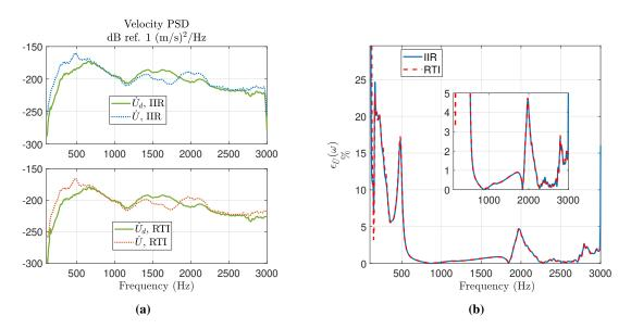
Fig. 20 Auto-PSDs of desired  $U_d$  and actual U velocity (a), and corresponding error percentage (b), obtained by targeting a linear SDOF dynamics of the ER with  $\mu_M = 1$ ,  $\mu_K = 2$  and  $R_{at} = \rho_0 c_0$  by either the IIR or the RTI.
