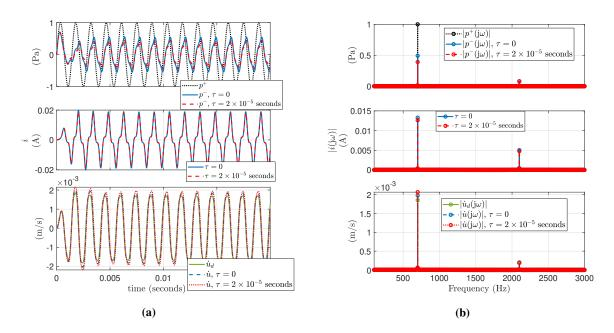
Fig. 8 Time histories (a) and DFTs amplitudes (b) of incident p and reflected  $p^-$  pressures, electrical current *it*, target  $u_d$  and actual u velocities, in case of Duffing desired dynamics of the ER. The excitation p is at 700 Hz. Both synchronous ( $\tau$  0) and delayed ( $\tau$  2 × 10<sup>-5</sup> seconds) simulation results, are showed.
