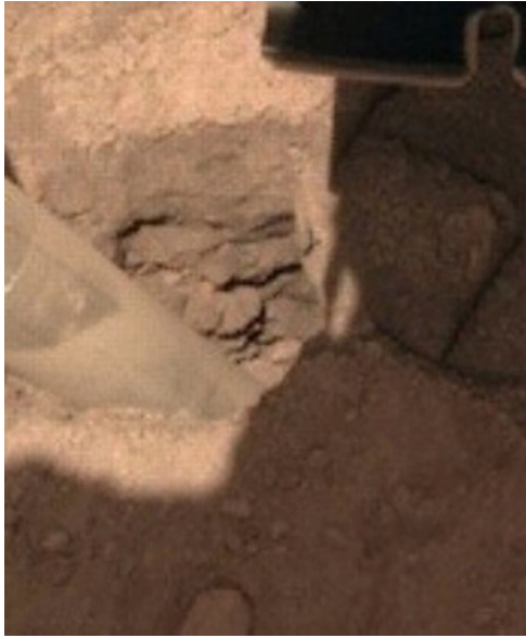
Figure 23. Image of the pit (7 cm deep, 5-6 cm wide) created by the HP3 mole during hammering (inclined \sim 15^\circ ), with the scoop appearing on top right (image credit JPL/NASA).
