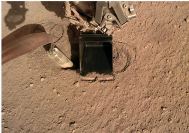
Figure 24. IDC photo showing the scoop of the IDA compressing the regolith with the mole (not in contact with the scoop, with the tether clearly visible) moved up during a reversal period (see Figure 20). The mole pit can be observed at the left of the scoop (image credit JPL/NASA).
