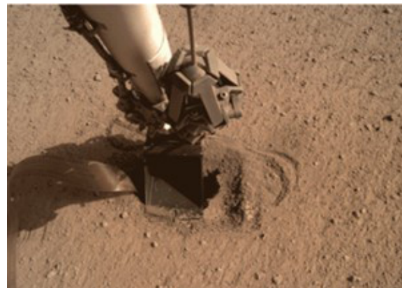
Figure 22. IDC photo showing the scoop of the Instrument Deployment Arm pressing on the mole during the Back Cap Push session, with the tether on the left side. The scoop is 7.6 cm in width and 10 cm in length (image credit JPL/NASA).
