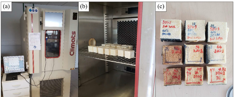
Fig. 4. (a) Climate chamber, (b) specimens during the ageing process, (c) specimens after ageing.
