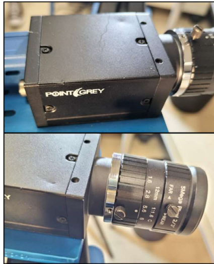
Fig. 6. Cameras used to capture the DIC images.
