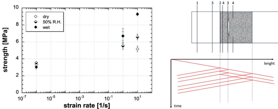
Fig. 15.22. Results of quasi-static and dynamic tests performed with concrete having 10mm aggregate size under dry, 50%R.H. and wet condition [Cadoni et al. 2001].
