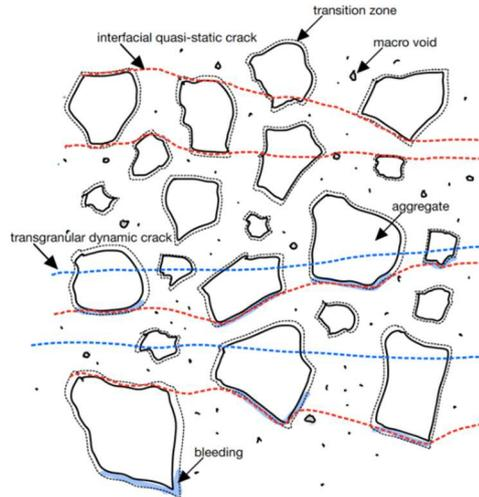
Figure 15.1 – Cracking pattern in quasi-static and dynamic regimes.
