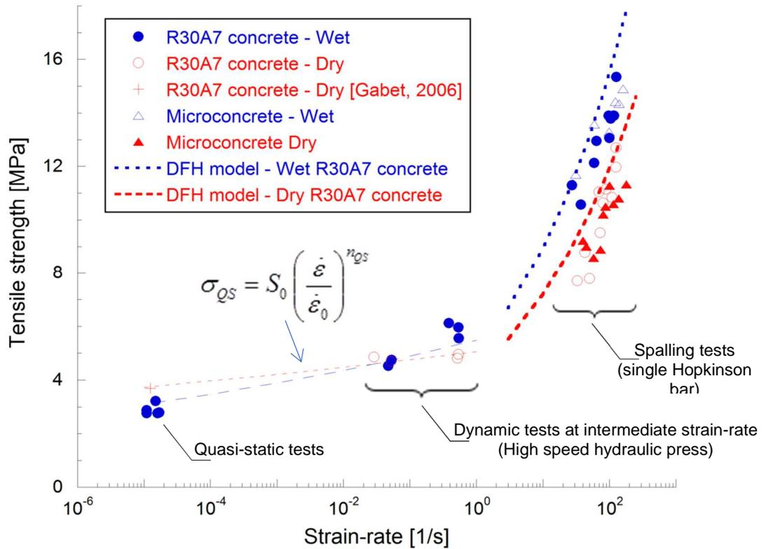
Fig. 15.21. Results of quasi-static and dynamic tests performed with MB50 and R30A7 concretes [Erzar and Forquin, 2011].
