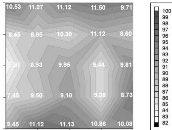
Figure 15.8 – Crack pattern and local strengths distribution over the cross-section of a concrete specimen during a tensile test @  $10 \text{ s}^{-1}$ .
