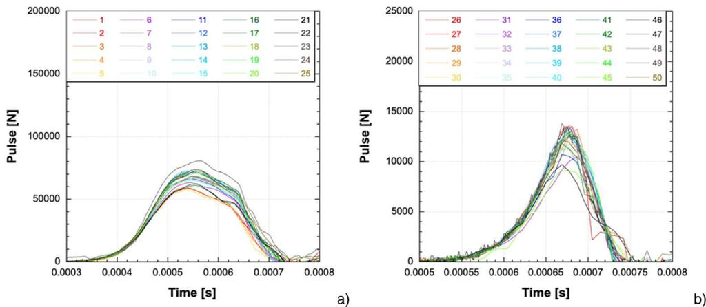
Fig. 15.5 – HBB experimental raw signals: a) input signals of the elementary bars; b) output signals of the elementary bars.
