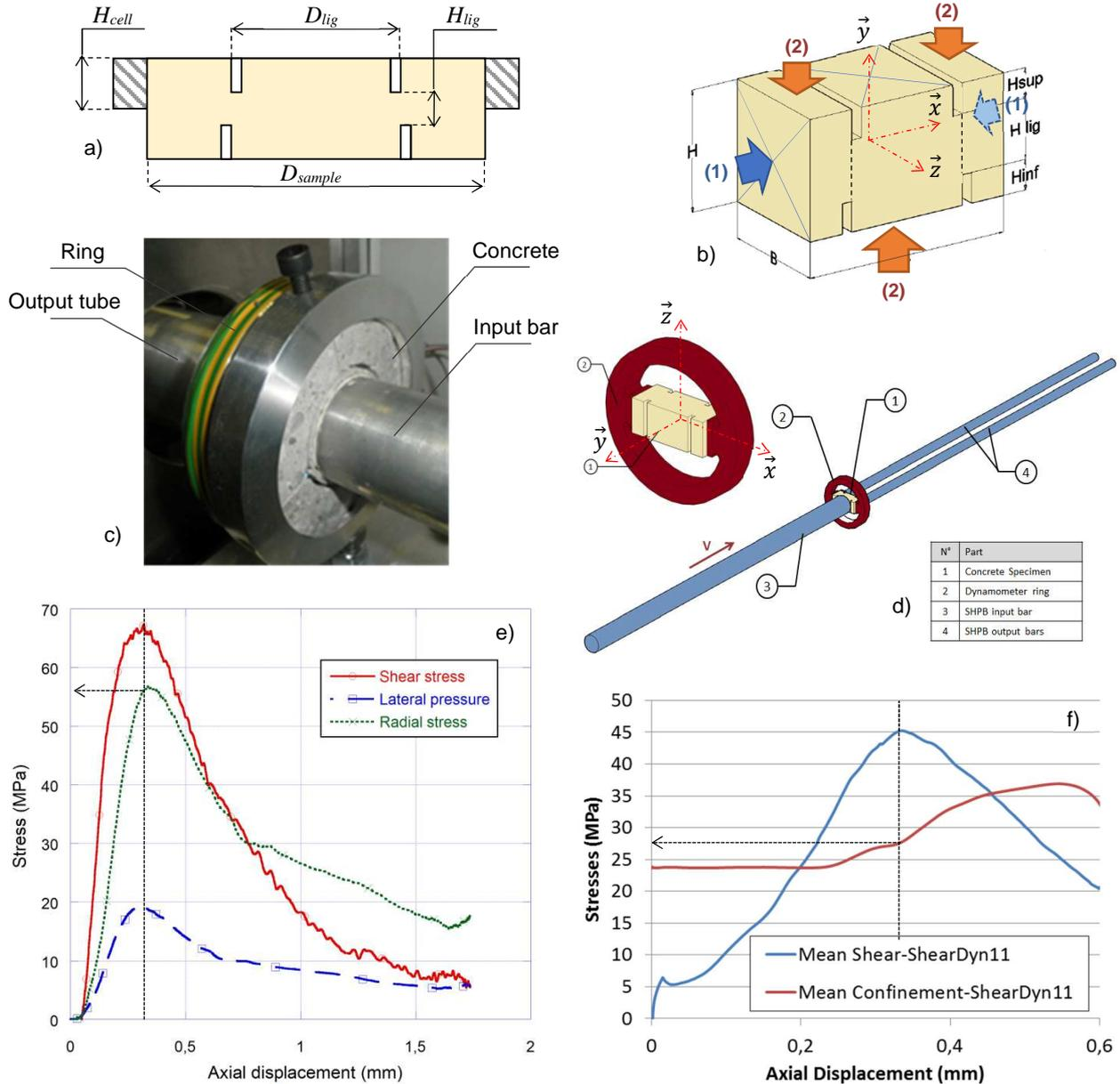
Figure 15.19 – Punch-Through-Shear (PTS) experiments performed in dynamic conditions. a) Oedo (oedometric)-PTS sample geometry, b) PS (Pre-Stressed)-PTS sample geometry, c) Oedo-PTS testing set-up, d) PS-PTS testing set-up, e) Example of oedo-PTS experimental result [Forquin, 2011], f) Example of PS-PTS experimental result [Abdul-Rahman et al, 2021].
