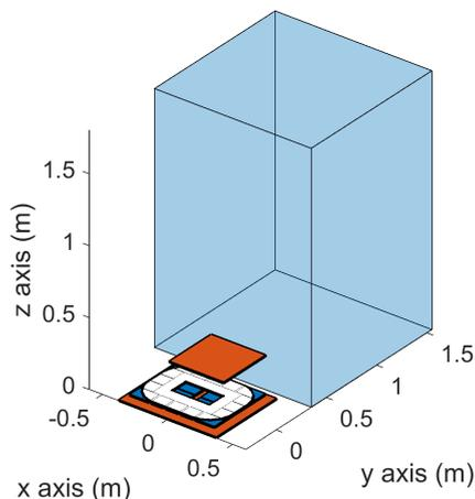
FIGURE 2: WPT3/Z3 system model from SAE J2954 (maximum misalignment between the coils) with an investigation volume (blue box of  $1.2 \text{ m} \times 1.2 \text{ m} \times 1.8 \text{ m}$  along the  $x$ ,  $y$  and  $z$  axis)
