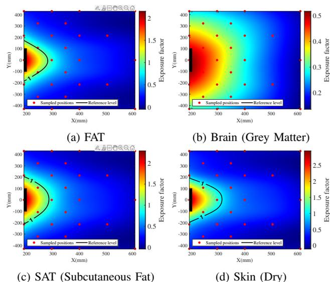
FIGURE 11: Variation of the exposure factor and safety area ( $I_{WP} < 1$ ) behind the MFDC welding gun for different tissues investigated in the case of general public exposure
