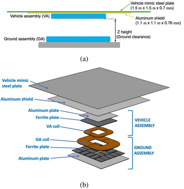
FIGURE 1: Cut plane (a) and 3D view (b) of the WPT3 (class Z3) system taken from from the SAE J2954 standard [25]
