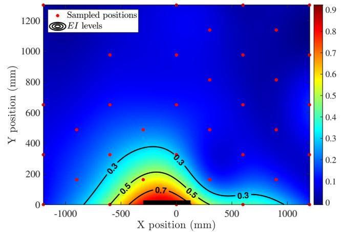
FIGURE 4: PCK metamodel ( $n_{samples} = 35$ ,  $LOO = 0.1945$ ) of  $EI_{\max}(x, y)$  for various positions of a crouched operator around the WPT3/Z3 system (black rectangle)
