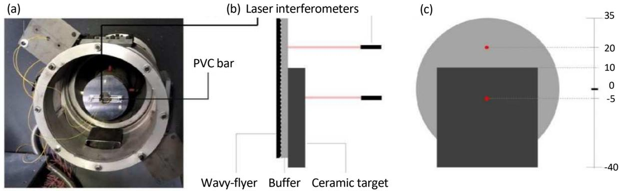
Fig. 17. (a) Instrumented rear face of the ceramic target. Schematic showing the 2 laser-probes set-up used to measure simultaneously the loading pulse and the ceramic free-surface velocity. Side view (b) and back view (c) (Dargaud and Forquin, 2022).
