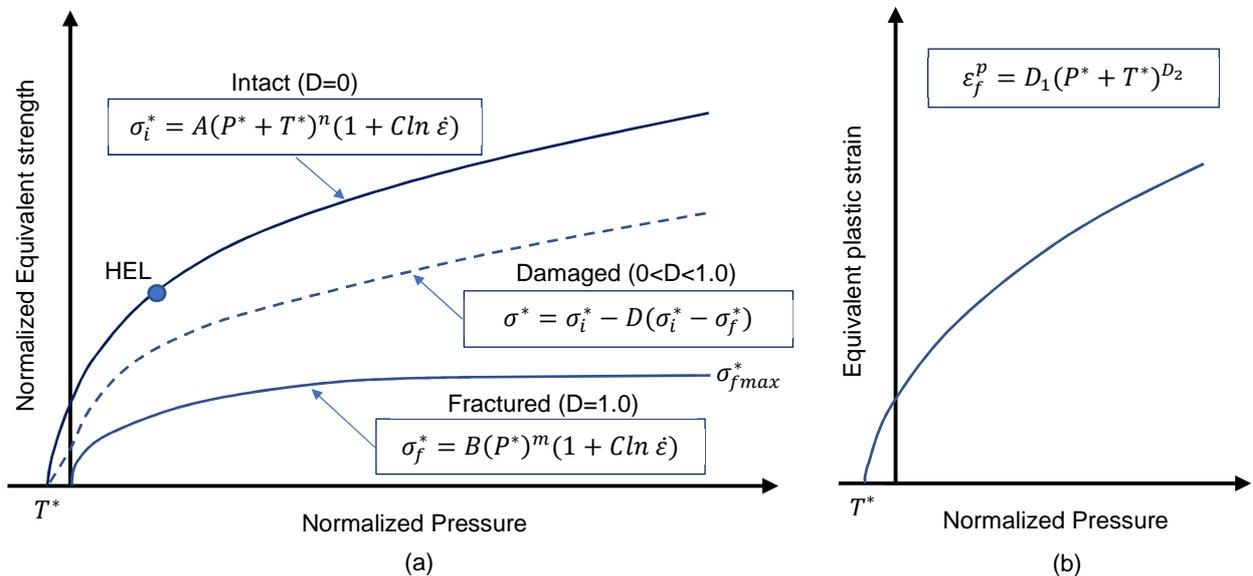
Fig. 22. The JH-2 plasticity-damage model. (a) Envelopes of intact and fractured material, (b) Damage evolution law.
