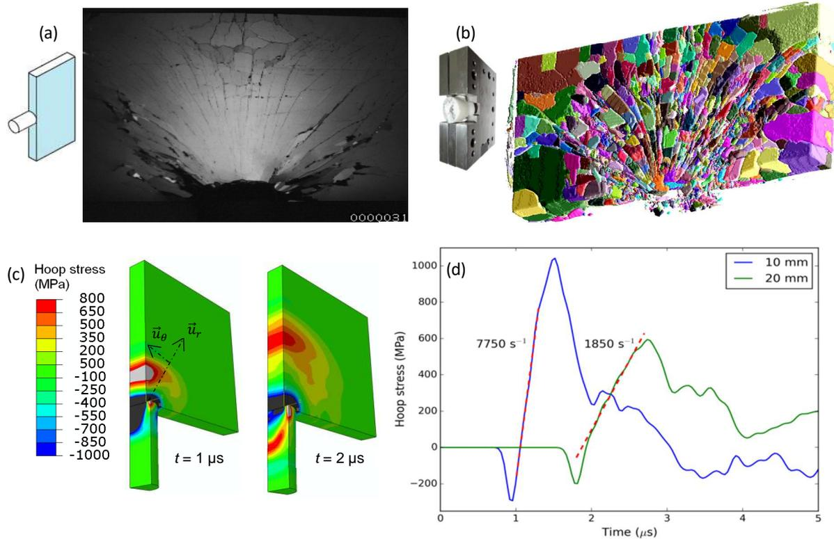
Fig. 16. The edge-on impact testing configuration. (a) EOI test conducted in open configuration and visualisation with an ultra-high-speed camera ( $t = 12 \mu\text{s}$ ) (Forquin et al, 2018), (b) EOI test performed in sarcophagus configuration and analysis of the fragment' size distribution with X-ray micro-tomography (Forquin and Ando, 2017), (c) Numerical simulation of EOI test and (d) traces of the hoop stress at 10 mm and 20 mm from the impact point (Forquin and Ando, 2017).
