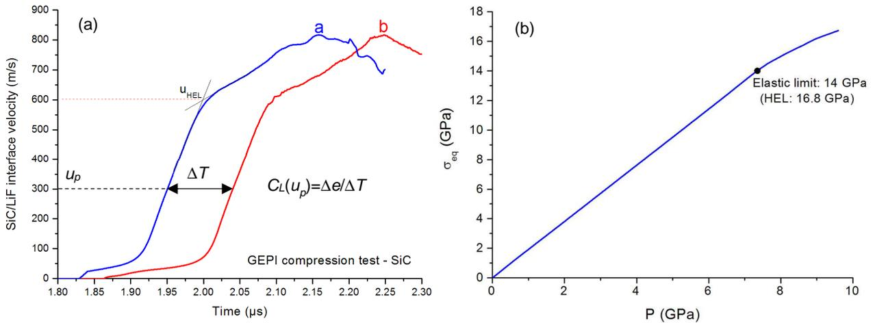
Fig. 14. Data processing GEPI compression test on two SiC specimens. (a) Velocity signals measured on two specimens with thicknesses  $e = 3$  and  $4$  mm (arbitrary origin of time). (b) Obtained response in terms of equivalent stress versus pressure.
