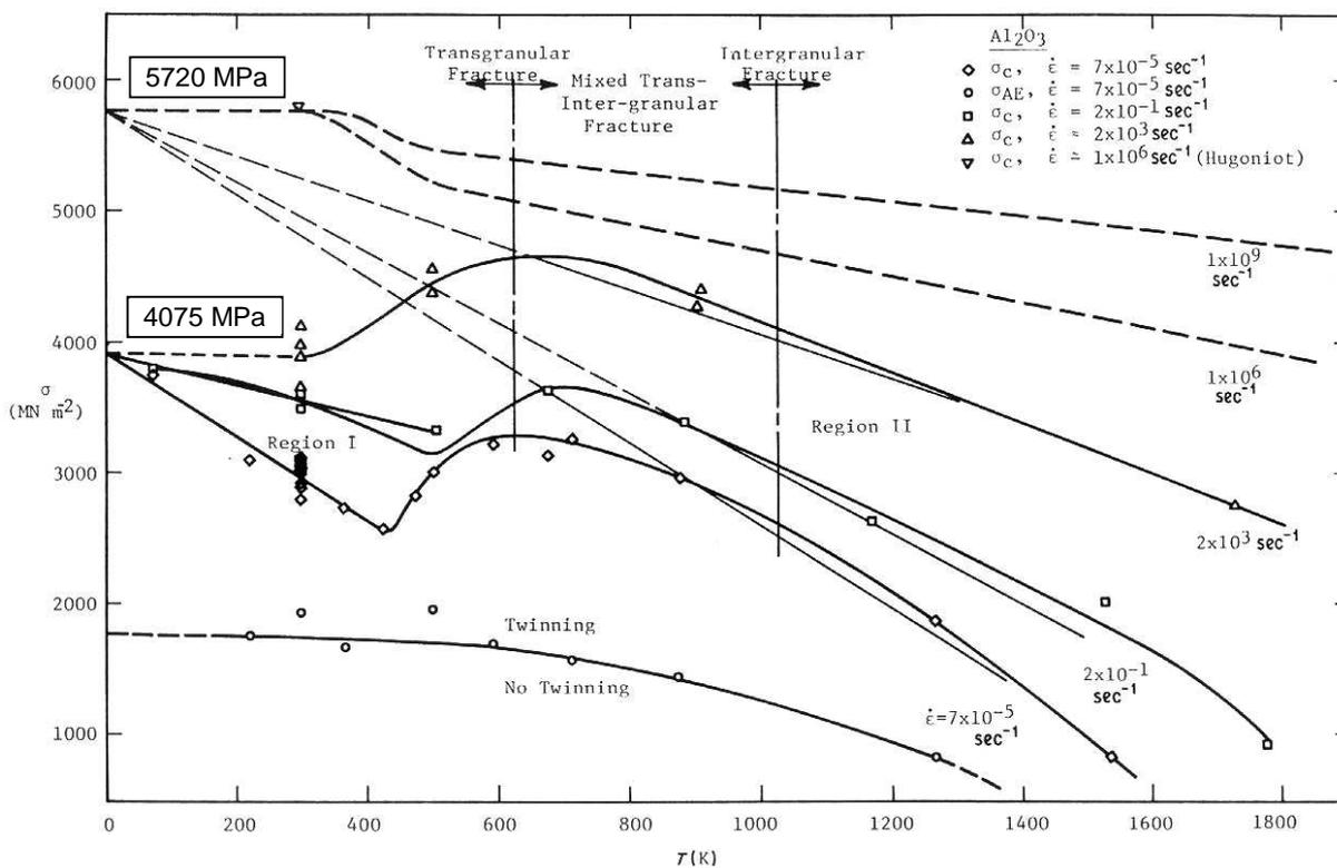
Fig. 7. Quasi-static uniaxial compression strength of alumina as a function of temperature (Lankford, 1981).
