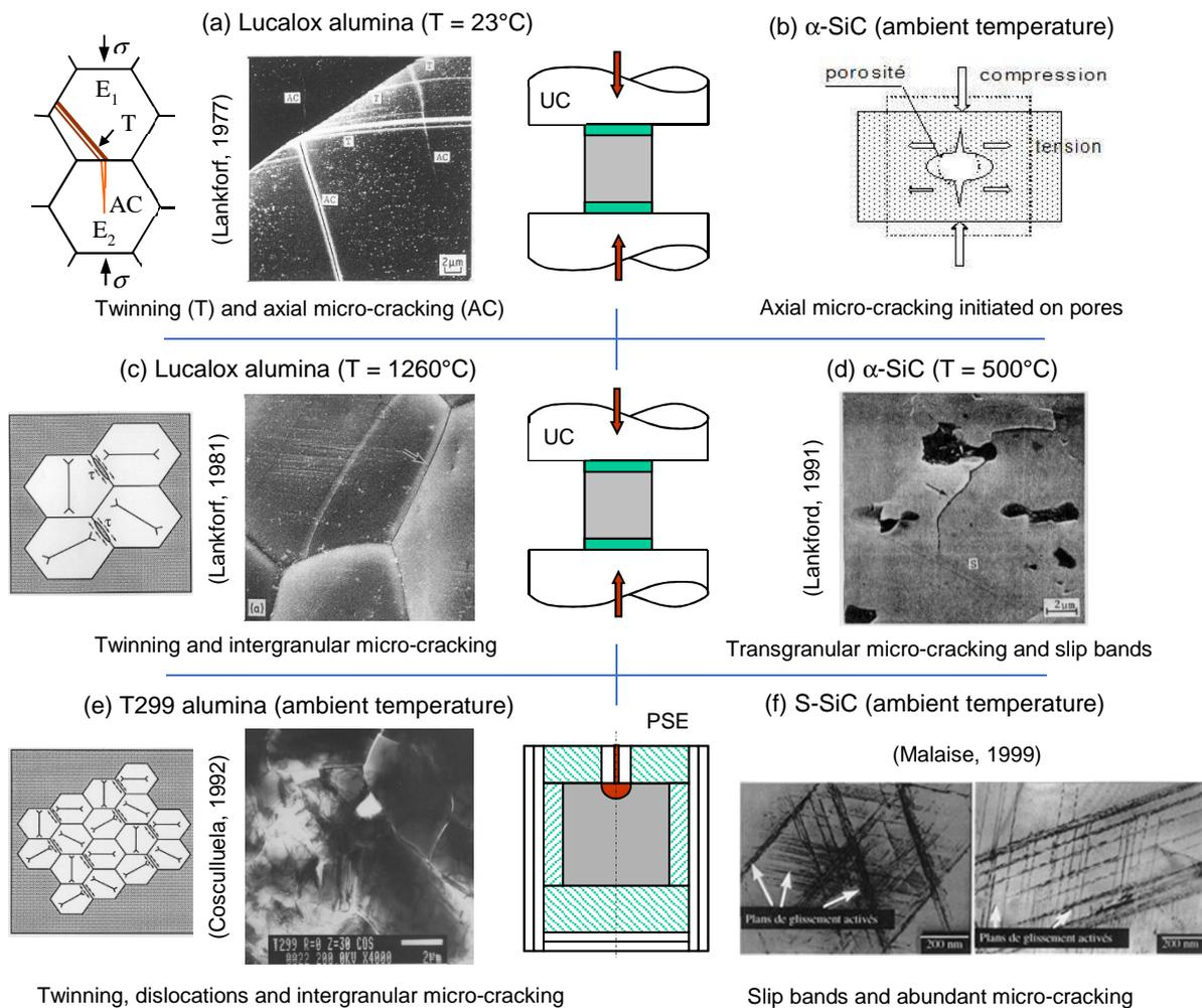
Fig. 8. Microplasticity and microcracking mechanisms observed in alumina and SiC ceramics under uniaxial compression (UC) test at ambient and elevated temperature and in pyrotechnic spherical expansion test (PSE) at ambient temperature. Figure derived from Forquin (2003) with illustrations from Lankford (1977; 1981; 1991), Coscolluela (1992) and Malaise (1999).
