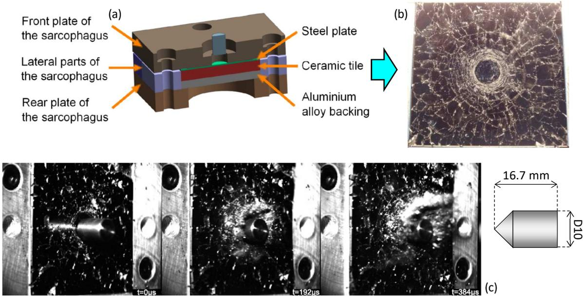
Figure 20. The tandem testing technique (Zinszner et al, 2015). (a) Normal impact against a sandwich configuration composed of a steel front plate, a ceramic tile and an aluminium backing plate. (b) Top view of the ceramic after normal impact. (c) Second impact with a conical-nose projectile at an impact speed of 175 m/s.
