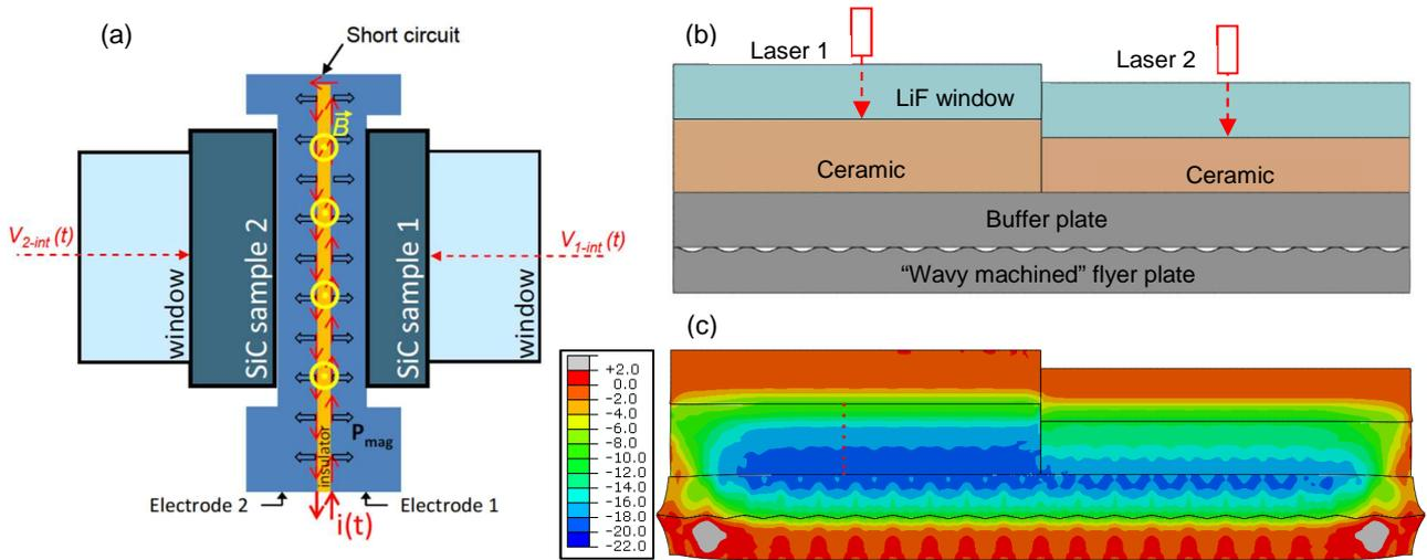
Fig. 13. Two experimental configurations used to perform compression tests which allow the use of Lagrangian analysis. (a) The GEPI facility (CEA-Gramat). (b) The shockless plate-impact configuration based on the wavy-machined flyer plate technique proposed in the 3SR Lab. (Grenoble).
