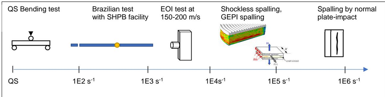
Fig. 19. Orders of magnitude of the strain-rate reached in samples subjected to various tensile loading tests.
