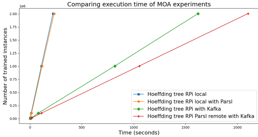
Fig. 7. Comparison of MOA local, MOA with Kafka and MOA with Remote Parsl and Kafka
