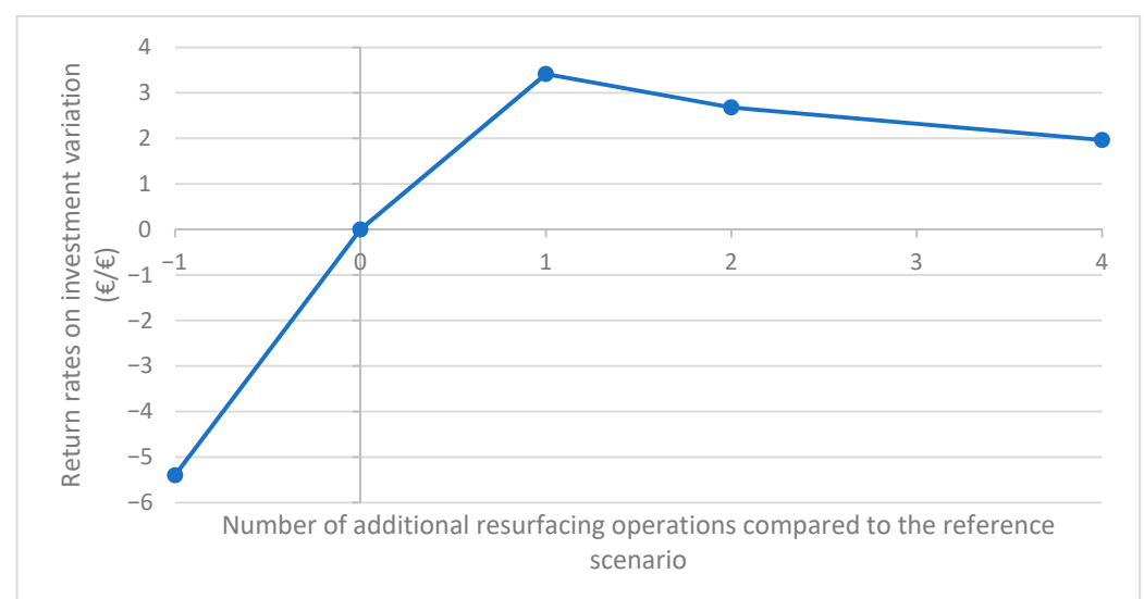
Figure 5. Users' savings for each additional euro invested in maintenance by the road operator (relative to the standard maintenance level).
