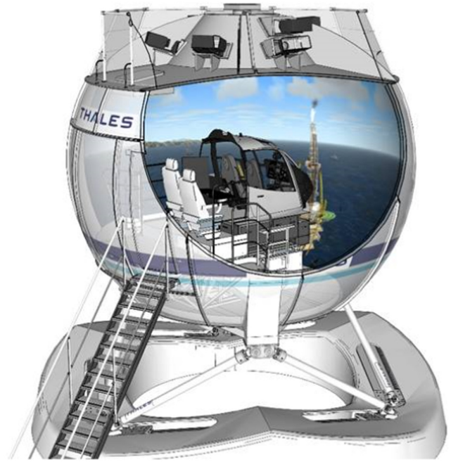
FIGURE 1 The EC135 cabin is in the display dome and the dome is over the six-degrees-of-freedom motion platform. The pilot is seated in the cabin.
