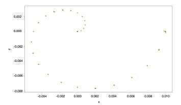
Fig. 6. Results obtained for the Liandford robot control for the first case: position on the x-z plane for the spiral trajectory. Green: the objective. Orange: position of the effector on the considering plane.
