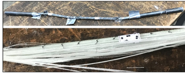
Figure 5: Typical tensile failure modes of GFRP (bottom) and CFRP (top) rebars, after exposure to ANL conditions.
