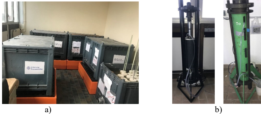
Figure 3 : a) Conditioning of ANL specimens in thermoregulated tanks filled with the alkaline solution; b) Metallic devices used for exposing the FRP specimens to an alkaline environment combined with sustained load (ASL conditions)
