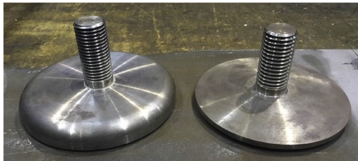
Fig. 2. Photo of studied fastener (tension on the left and shearing on the right) [4]
