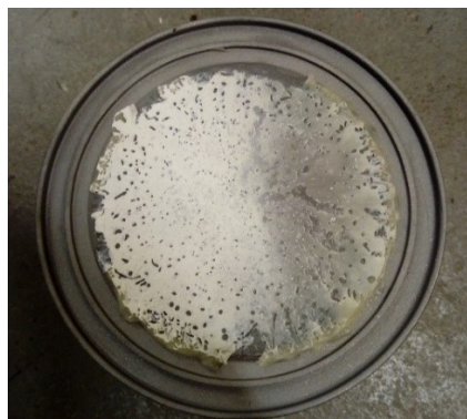
Fig. 5. Photo of the fracture surface of a creep shear test at 65% of S_{ult}
