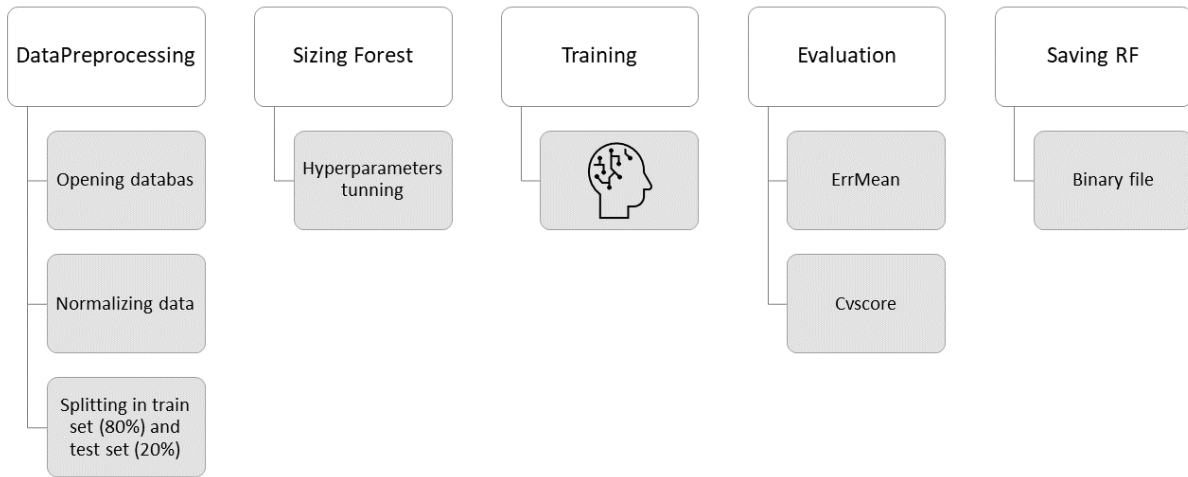
Figure 8: Workflow of machine learning processing
