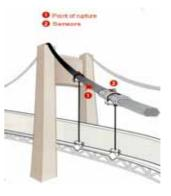
Figure 1: Rupture detection by acoustic sensors
