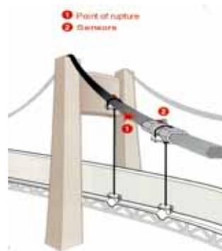
Figure 1: Rupture detection by acoustic sensors
