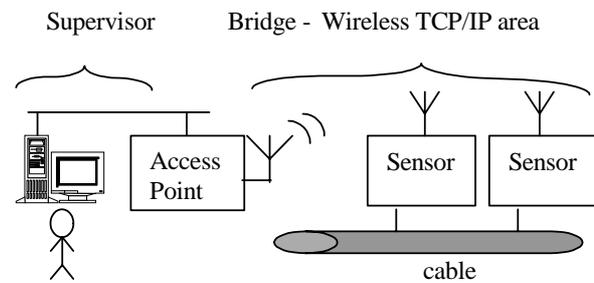
Figure 5: The wireless sensor network architecture
