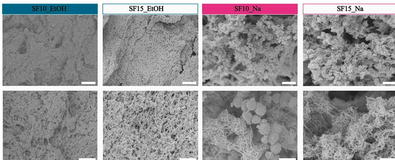
Fig. 4. SEM images of SF (10 and 15 %w/v) aerogels prepared after coagulation in ethanol or  $\text{NaH}_2\text{PO}_4$  solution. Scale bar low magnification (top) 2  $\mu\text{m}$ ; scale bar high magnification (bottom) 500 nm.
