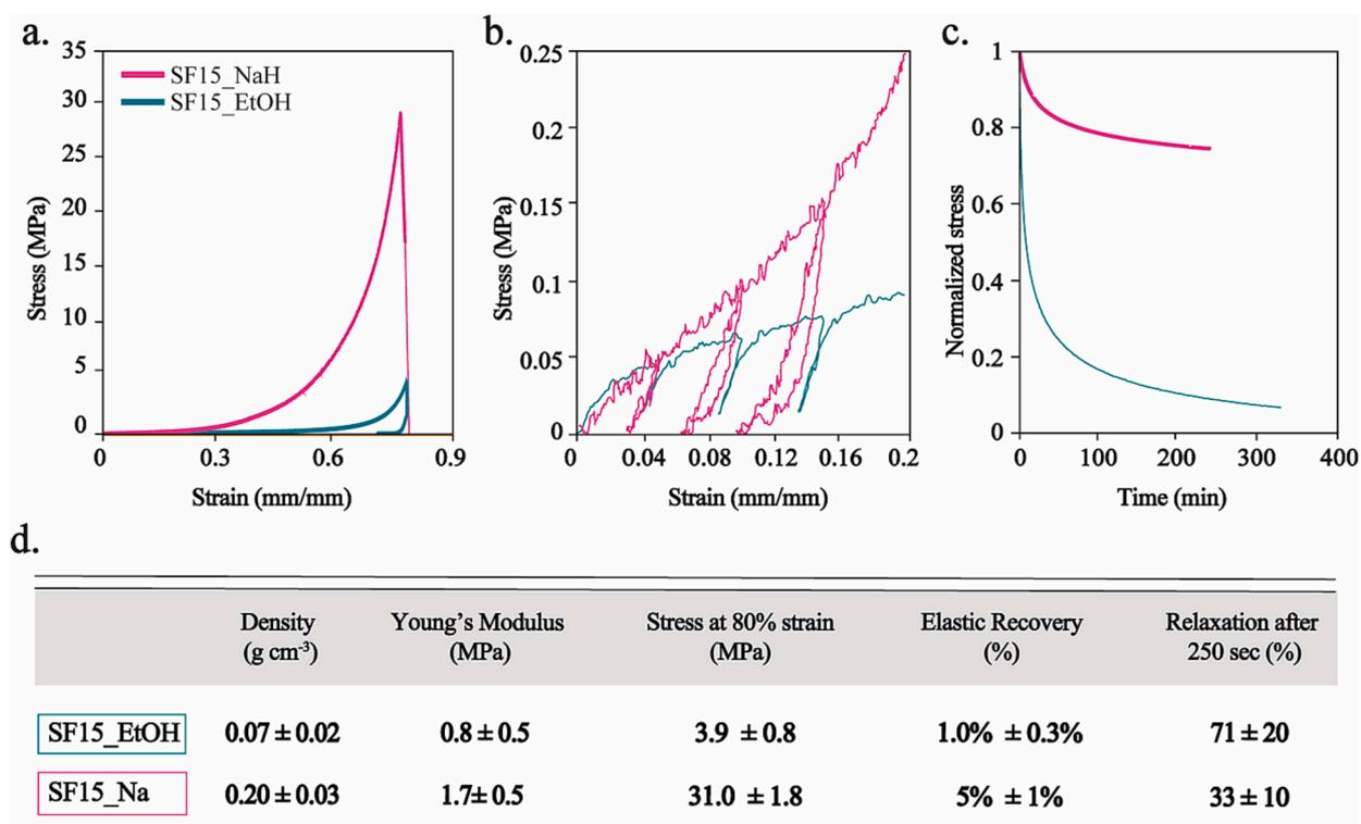
Fig. 5. (a) Nominal stress–strain full curves and (b) at low strains for SF15\_Na and SF15\_EtOH aerogels; (c) Relaxation curves after stopping compression for SF15\_Na and SF15\_EtOH aerogels; (d) Main characteristics of SF aerogels: Young's modulus, stress at 80% strain, elastic recovery and relaxation after 250 s.
