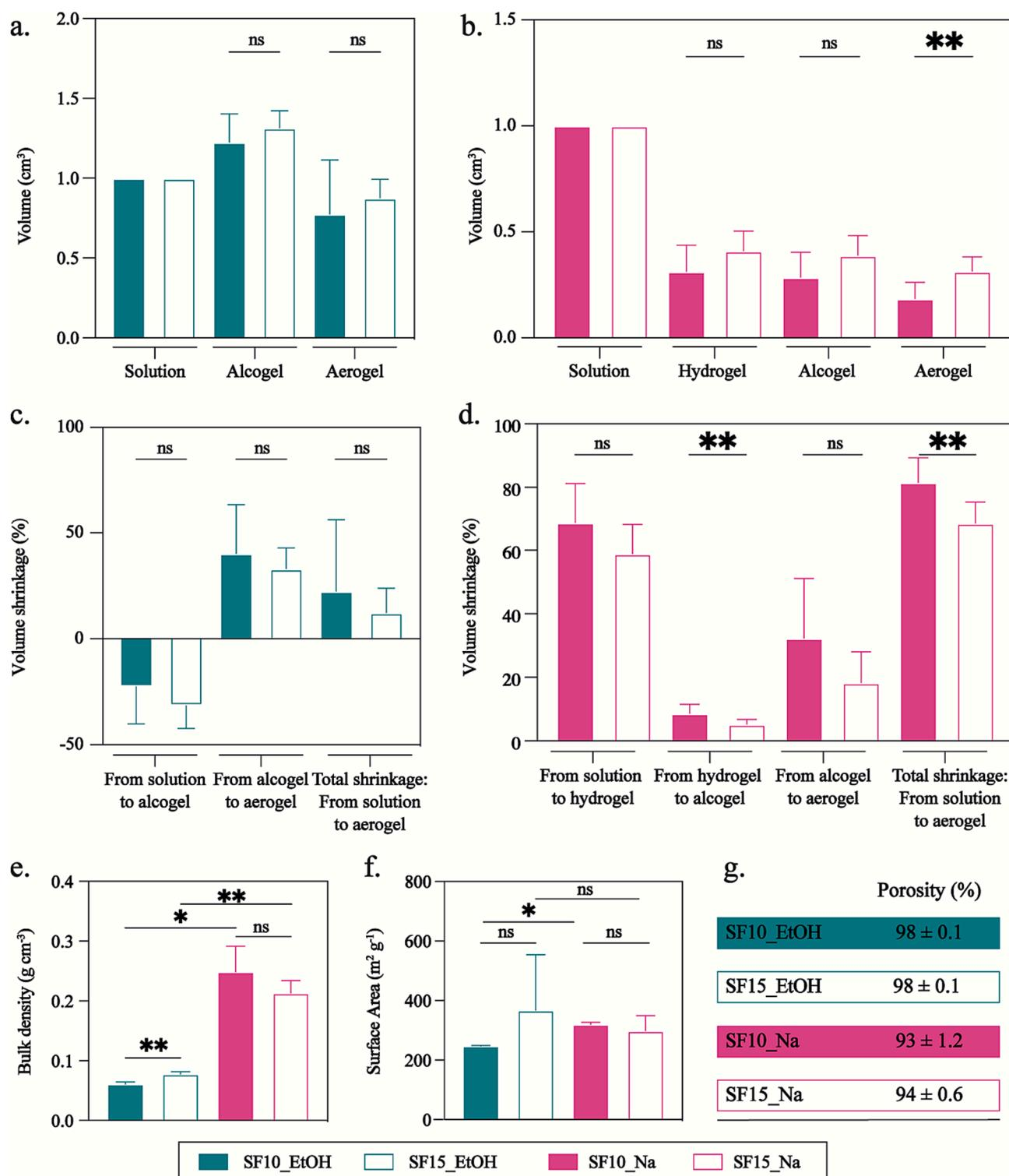
**Fig. 3.** Characteristics of all SF samples, (a, c) for Method 1 and (b, d) for Method 2: (a, b) Volume at every stage of the process, from solution to aerogel (\*\* =  $p < 0.01$ ); (c, d) shrinkage (\* =  $p < 0.05$ ; \*\* =  $p < 0.01$ ); (e) density (\* =  $p < 0.05$ , \*\* =  $p < 0.01$ ,  $n = 3$ ); (f) specific surface area (\*\* =  $p < 0.01$ ,  $n = 3$ ); (g) porosity.
