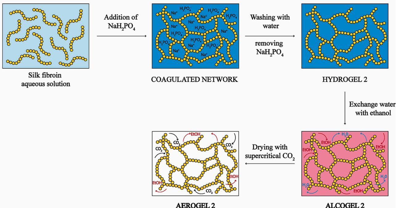
Fig. 1. Schematic presentation of two methods of SF aerogels preparation: Method 1 - via direct coagulation in ethanol and Method 2 - via coagulation in NaH<sub>2</sub>PO<sub>4</sub>.
