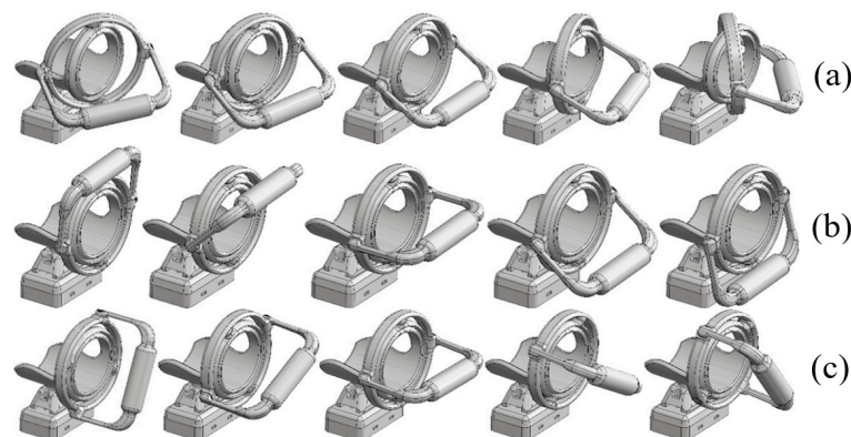
Figure 13. Simulations of VARONE’s motion, (a) UR deviation, (b) wrist FE, (c) forearm pronosupination.
