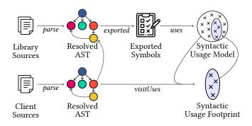
Figure 1: UCov parses and analyses Java code to build SUM and SUF models. Each cross symbol (×) represents one possible use of an API symbol.
