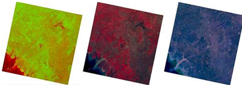
Fig. 4 Colour composites of the Landsat images covering study area: Left: false colour composite with aerosol channel (7-5-1); centre: false colour composite (bands 5-4-3) right: natural colour composite (bands 4-3-2)
