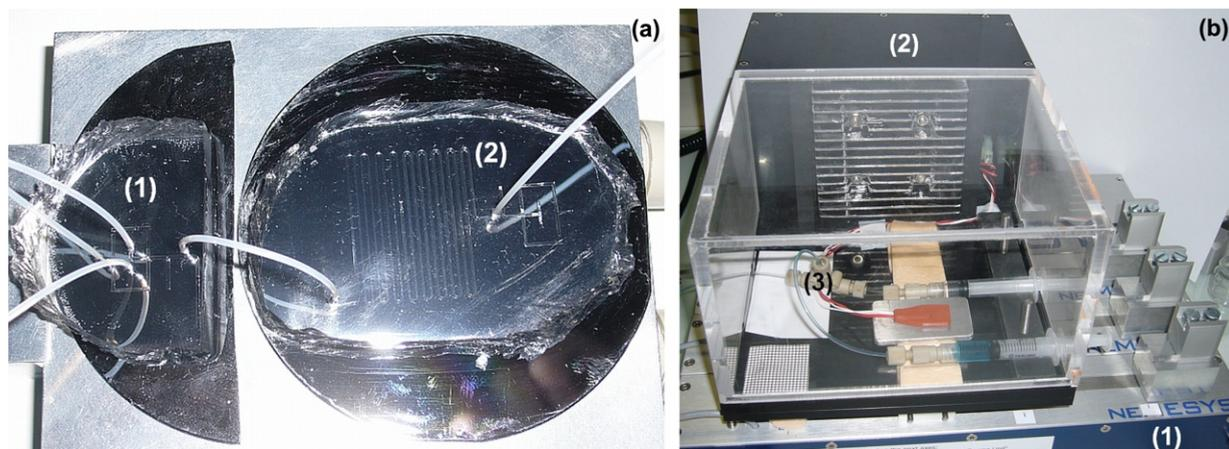
**Fig. 1.** (a) PDMS microfluidic device, (1) plug-factory and (2) droplet-storage zone, and (b) PEEK/Teflon microfluidic device, (1) syringe pumps, (2) temperature controller (room  $T$  to 60 °C) and (3) T-junction.
