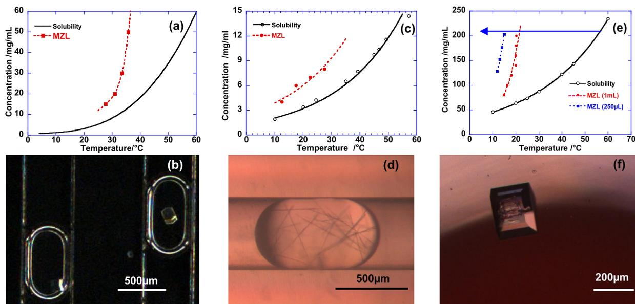
**Fig. 3.** Solubility and MZ limit, (a) lysozyme in NaCl 0.7 M and pH = 4.5 (device in PDMS), (c) caffeine in ethanol (device in PEEK/Teflon) after [18] with permission of ACS and (e) isonicotinamide in ethanol (multiwell of 1 mL and 250  $\mu$ L). (b) Lysozyme crystals in aqueous droplets, (d) caffeine crystals in ethanol droplet and (f) crystal of isonicotinamide in ethanol. For experimental procedures see Refs. [7,18,21].
