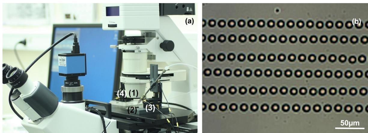
**Fig. 2.** (a) Image of the whole experimental nanofluidic set-up, (1) microscope, (2) glass micropipette, (3) XYZ miniature translation stages for injector and (4) sharp tungsten tip, and (b) array of monodisperse water droplets (11.8  $\mu\text{m}$  or 0.7  $\mu\text{L}$ ).
