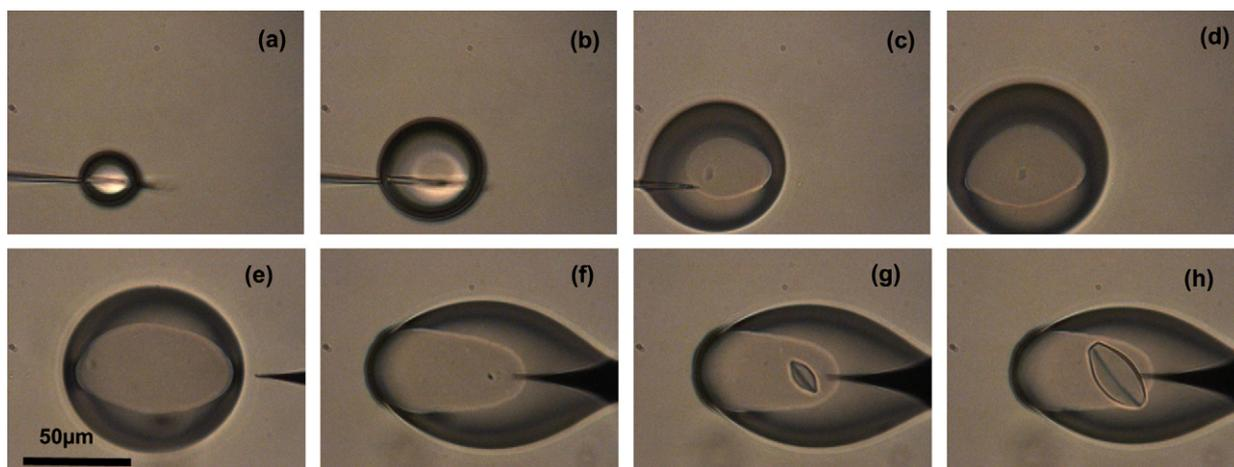
**Fig. 5.** ((a) to (d)) Generation of a BPTI droplet (20 mg/mL) in NaCl (1.6 M) in DMS oil and nucleation and growth of BPTI, (e) droplet size 85  $\mu\text{m}$  (200 pL) at  $t = 0$ , (f)  $t = 30$  min, (g)  $t = 80$  min and (h)  $t = 130$  min.
