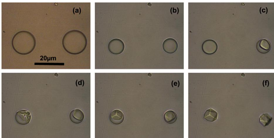
**Fig. 4.** Nucleation and growth of  $\text{KNO}_3$  (1.9 M) in  $\text{H}_2\text{O}$  in FC-70 oil, (a) droplet size  $15 \mu\text{m}$  (2 pL) at  $t = 0$ , (b) droplet size  $9.3 \mu\text{m}$  (0.48 pL),  $t = 8 \text{ min } 29 \text{ s}$ , (c)  $t = 9 \text{ min } 15 \text{ s}$ , (d)  $t = 9 \text{ min } 17 \text{ s}$ , (e)  $t = 10 \text{ min } 18 \text{ s}$  and (f)  $t = 12 \text{ min } 12 \text{ s}$ .
