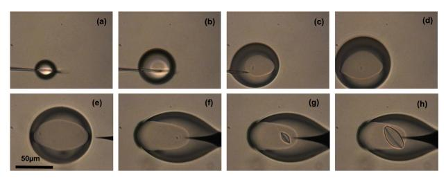
**Fig. 5.** ((a) to (d)) Generation of a BPTI droplet (20 mg/mL) in NaCl (1.6 M) in DMS oil and nucleation and growth of BPTI, (e) droplet size 85  $\mu$ m (200 pL) at t = 0, (f) t = 30 min, (g) t = 80 min and (h) t = 130 min.
