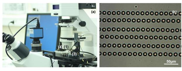
**Fig. 2.** (a) Image of the whole experimental nanofluidic set-up, (1) microscope, (2) glass micropipette, (3) *XYZ* miniature translation stages for injector and (4) sharp tungsten tip, and (b) array of monodisperse water droplets (11.8 μm or 0.7 pL).
