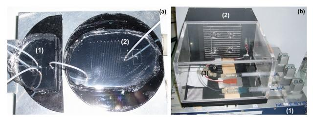
**Fig. 1.** (a) PDMS microfluidic device, (1) plug-factory and (2) droplet-storage zone, and (b) PEEK/Teflon microfluidic device, (1) syringe pumps, (2) temperature controller (room *T* to 60 °C) and (3) T-junction.
