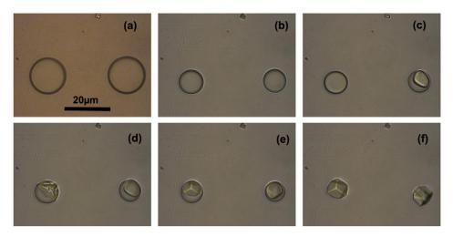
**Fig. 4.** Nucleation and growth of KNO<sub>3</sub> (1.9 M) in H<sub>2</sub>O in FC-70 oil, (a) droplet size 15  $\mu$ m (2 pL) at t = 0, (b) droplet size 9.3  $\mu$ m (0.48 pL),  $t = 8 \min 29 \text{ s}$ , (c)  $t = 9 \min 15 \text{ s}$ , (d)  $t = 9 \min 17 \text{ s}$ , (e)  $t = 10 \min 18 \text{ s}$  and (f)  $t = 12 \min 12 \text{ s}$ .
