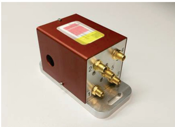
Figure 3. Multi-transducer VIS AOTF obtained at AA Opto Electronic.
