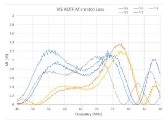
**Figure 6.** Mismatch Loss (in dB) for all five transducer setups in the applicable RF frequency range. Tr1 = leftmost transducer (2 mm), Tr2 = second from the left transducer (2 mm), Tr3 = middle transducer (3 mm), Tr4 = second from the right transducer (2 mm), Tr5 = right transducer (2 mm).
