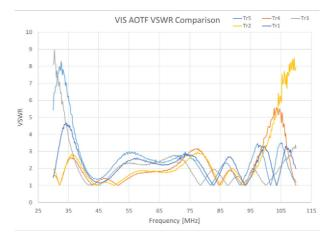
**Figure 5.** VSWR comparison graph for all five transducer setups. Tr1 = leftmost transducer (2 mm), Tr2 = second from the left transducer (2 mm), Tr3 = middle transducer (3 mm), Tr4 = second from the right transducer (2 mm), Tr5 = right transducer (2 mm).
