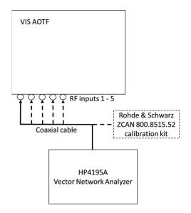
**Figure 4**. Test setup in order to characterize the different transducer setups of the VIS AOTF.
