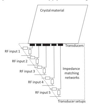
**Figure 2**. VIS AOTF transducer setups (= transducer – impedance matching network combinations).
