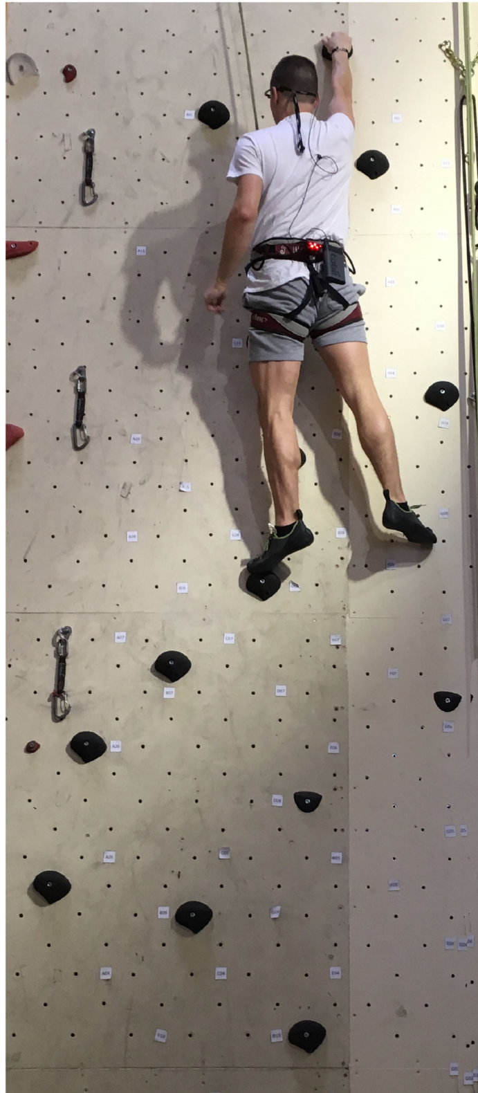
FIGURE 2 Climbing route setup: the led lamp light to track the trajectory of the climber is attached to the harness along with the IMU. The handholds on the artificial wall are equipped with sensors.
