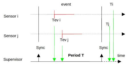
Figure 5 : synoptic of supervisor/sensors exchange.
