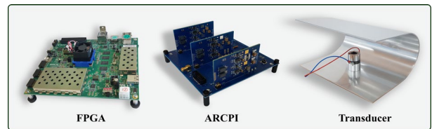
Fig. 12. Experimental setup of the ARCP Inverter.
