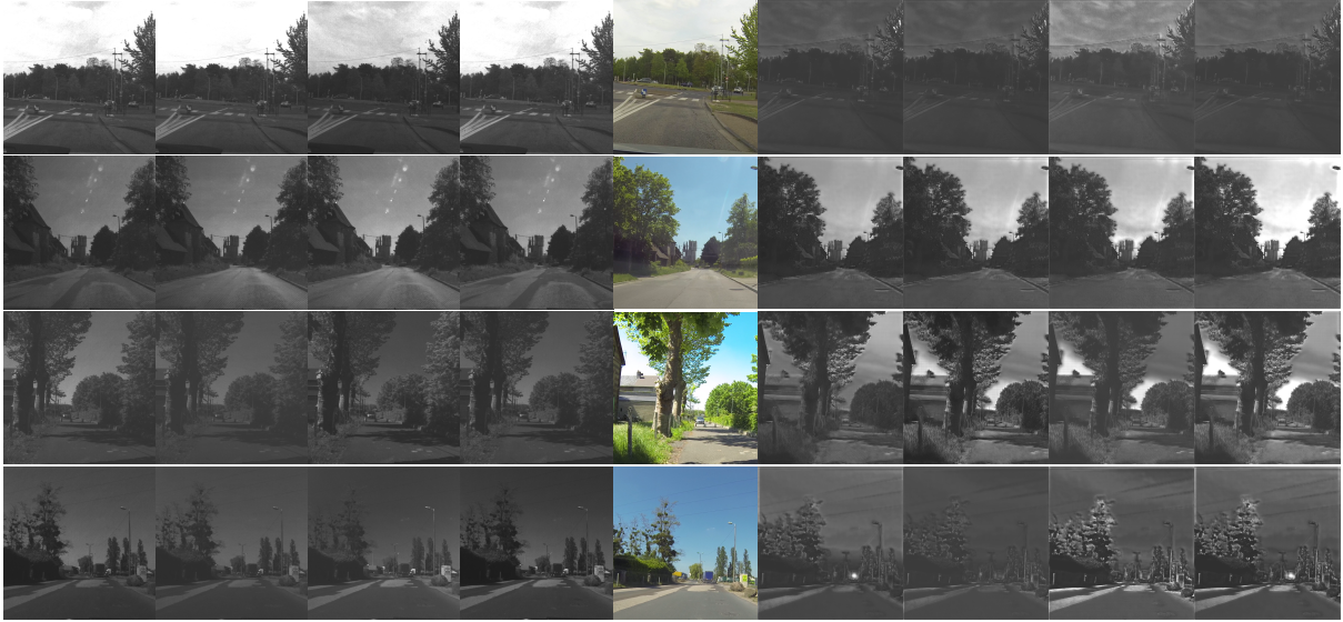
Figure 7: Examples of generated polarimetric images. From left to right: I_0, I_{45}, I_{90}, I_{135} (ground truth), RGB image and I_0, I_{45}, I_{90}, I_{135} generated from RGB.
