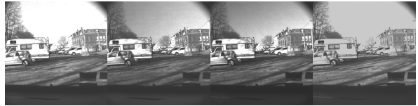
Figure 3: Example of a polarimetric image. From left to right, the intensities corresponding to the polarizer rotation angles 0^\circ, 45^\circ, 90^\circ and 135^\circ .
