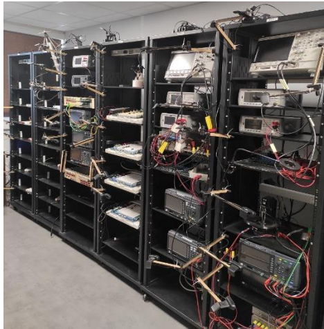
Fig. 2. Our remote lab based on 19", 42U racks shelves.
