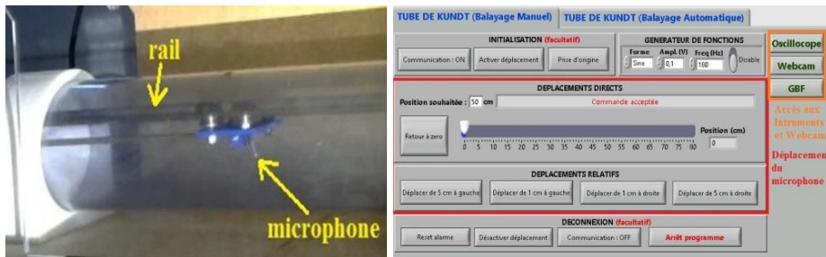
Fig. 6. Kundt experiment (left) and its Labview Interface (right)
