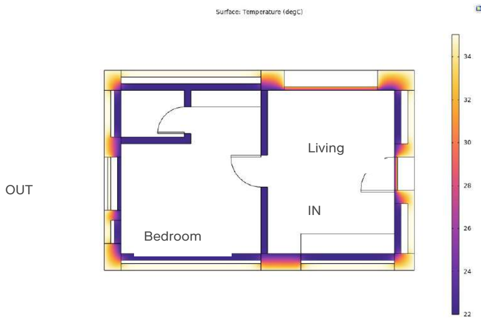
Figure 6. Heat transfer through double-wall concrete building envelope for peak summer temperature in Mediterranean climatic zone. Simulation by Authors using COMSOL Multiphysics® version 6.0 (drawing is not at scale)
