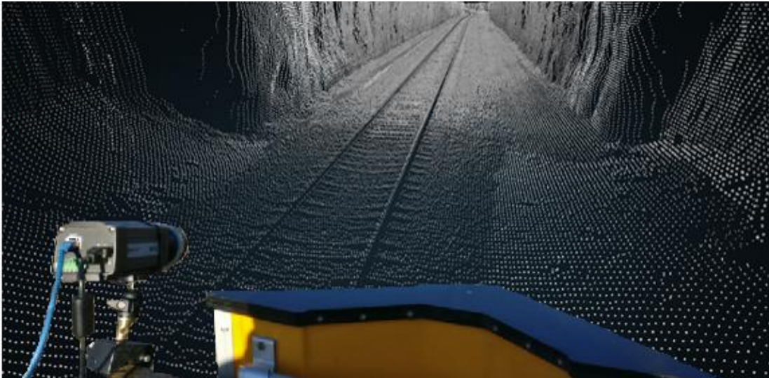
Figure 32. 3D GPR and thermal camera survey illustration in point cloud model from 2D laser scanner (Silvast et al., 2019).
