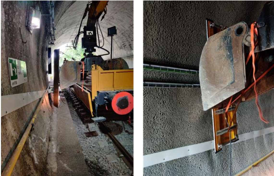
Figure 33. The GPR antenna DX1821 from 3D-radar attached to a shovel of an excavator on the flatcar (Silvast et al., 2021).
