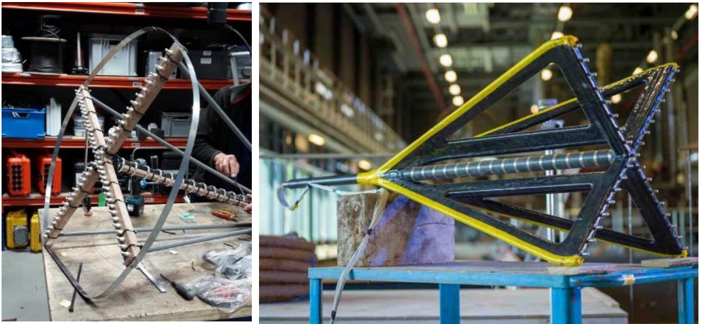
Figure 18. Left: prototype for experiments in water. Right: prototype for experiments in sand and clay. There are electrodes in the pole and on the two “forks” at the end of the pole. (Image: Deltares)
