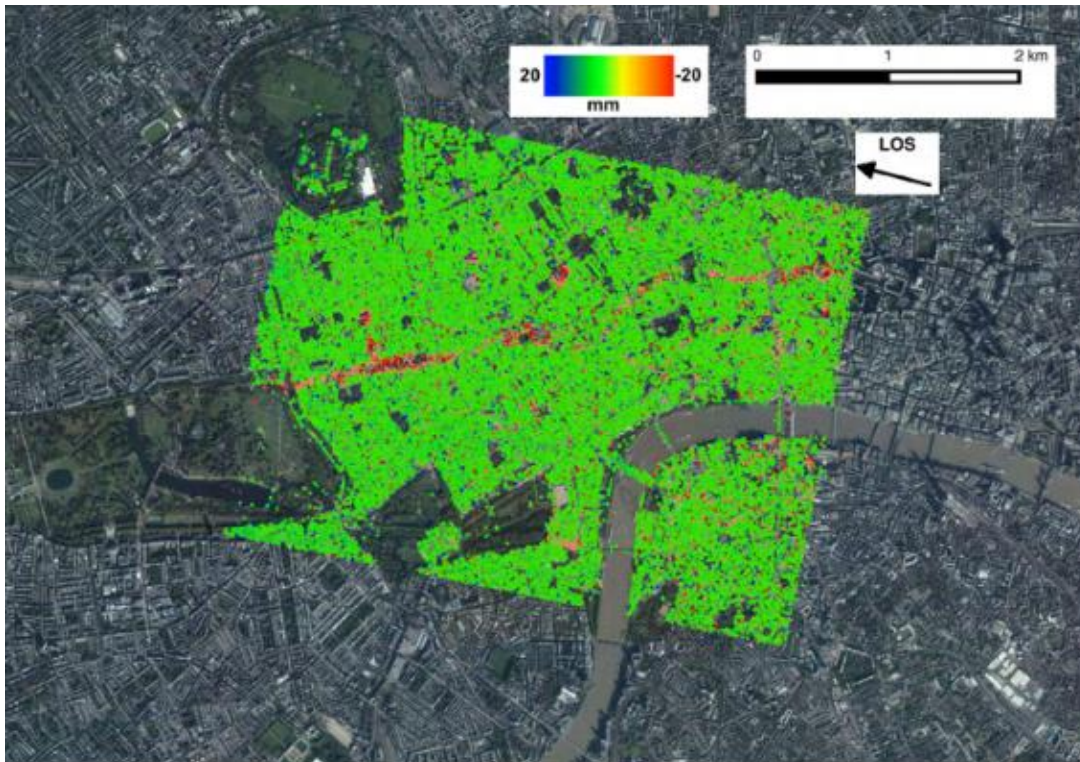
Figure 7. Cumulative displacement map over London spanning April 2011–December 2015 (Giardina et al., 2019). Negative values indicate targets moving away from the satellite. Blue stars indicate the locations of the analysed buildings.
