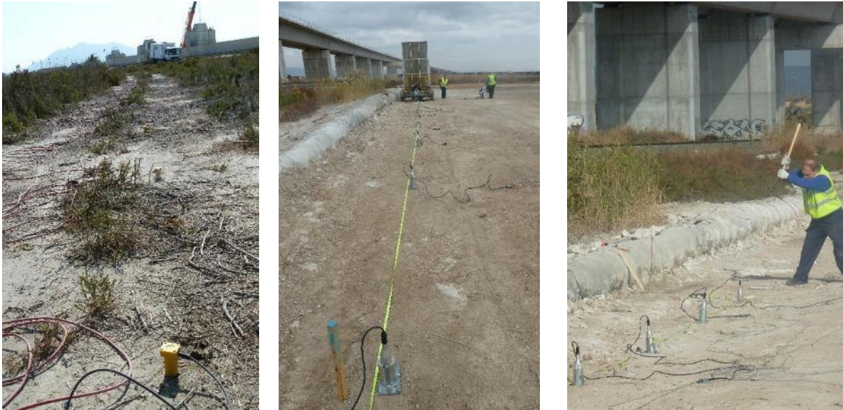
Figure 25. Seismic refraction (left), SASW (center), and free field transfer function (right)(Image: CEDEX)
