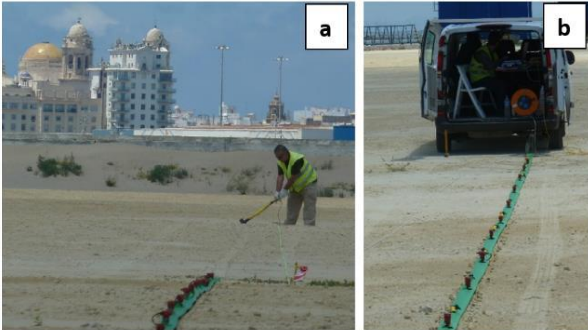
Figure 23. MASW test data acquisition. (a) Source and sensors array. (b) Sensors array. (Image: CEDEX)
