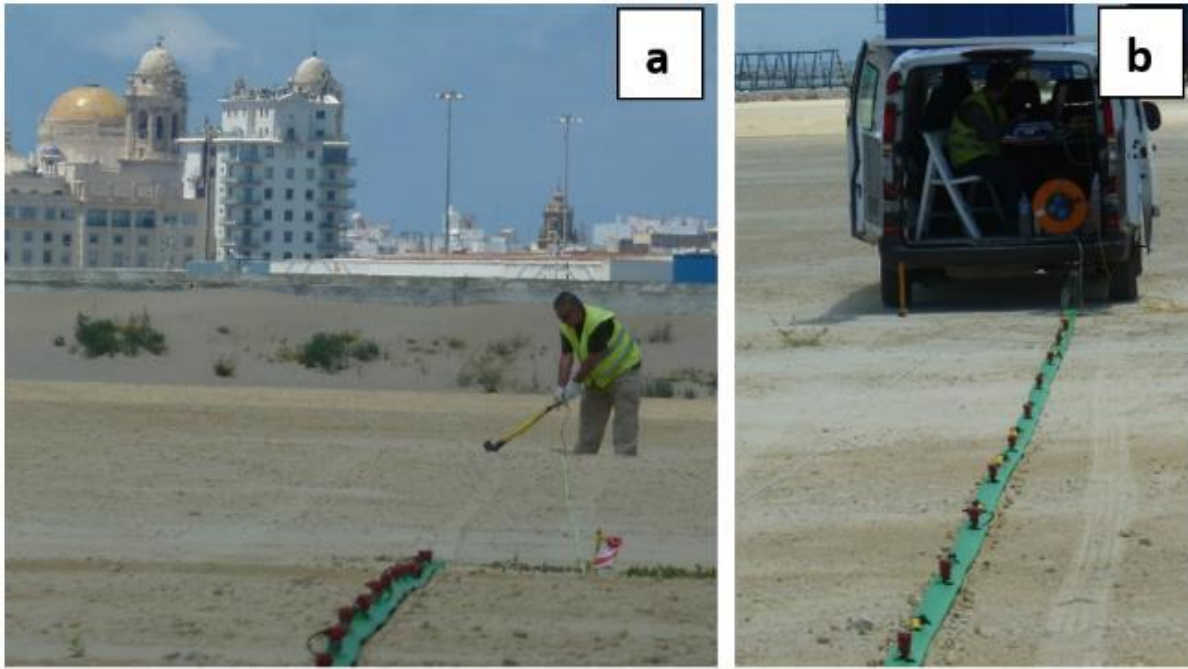
Figure 23. MASW test data acquisition. (a) Source and sensors array. (b) Sensors array. (Image: CEDEX)
