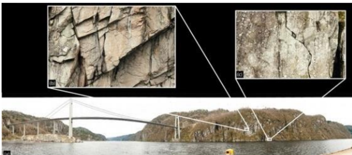
Figure 14. GigaPan imaging technology generates a panorama with extremely high resolution (Fedafjorden and Flekkefjord) to supplement LiDAR-data (Image: NGI)
