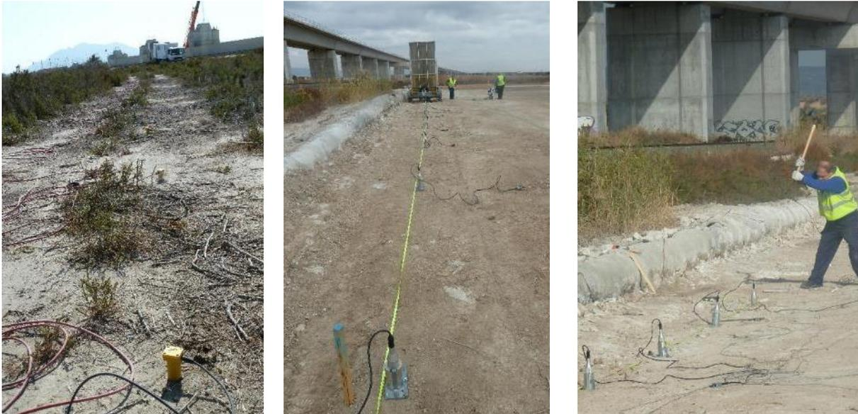
Figure 25. Seismic refraction (left), SASW (center), and free field transfer function (right)(Image: CEDEX)
