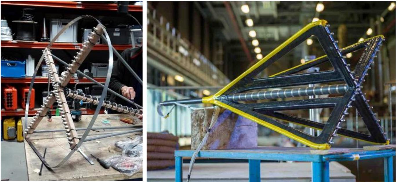
*Figure 18. Left: prototype for experiments in water. Right: prototype for experiments in sand and clay. There are electrodes in the pole and on the two “forks” at the end of the pole. (Image: Deltares)*
