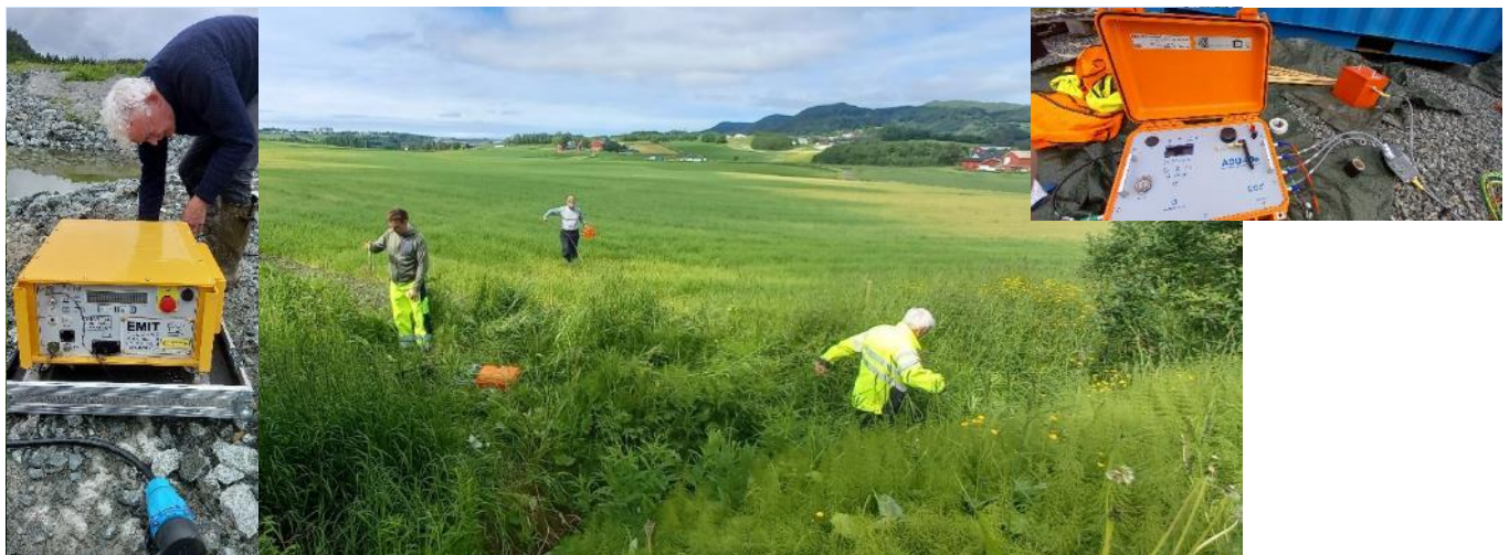
Figure 36. Equipment and ground investigation with ground-based EM survey conducted in June 2022 at the Tiller-Flotten test site. The research is within GEOLAB- Transnational Access project QC-CEM with user group from Luleå University (Photo: Olger Gjuzi)
