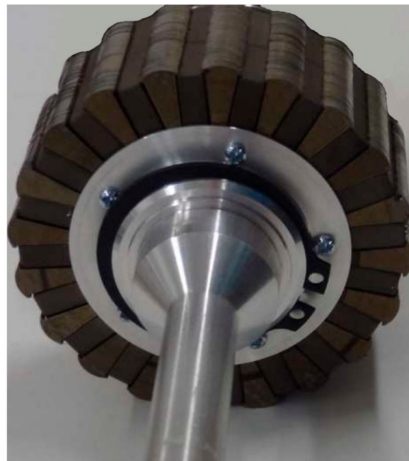
Figure 5. View of the designed through shaft.
