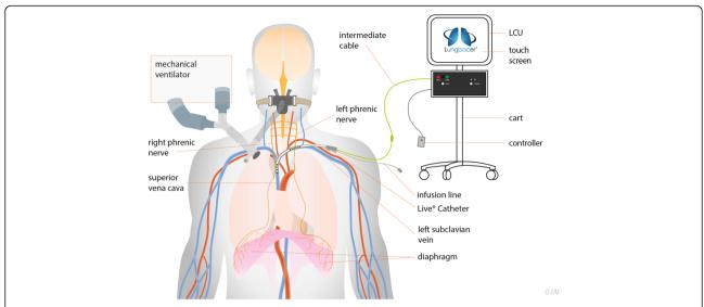
Fig. 2 Schematic representation of the Lungpacer LIVE® Catheter system providing temporary transvenous phrenic stimulation for diaphragm pacing (LCU Lungpacer Control Unit). Credit to Mr. Jean Allard
