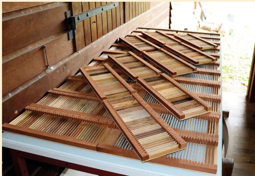
Photo 1. The 445 samples used to measure the modulus and the damping coefficient. The manufacturing of custom-made storage racks limits the risk of error and optimizes the handling of the samples. Photo J. Beauchêne.
