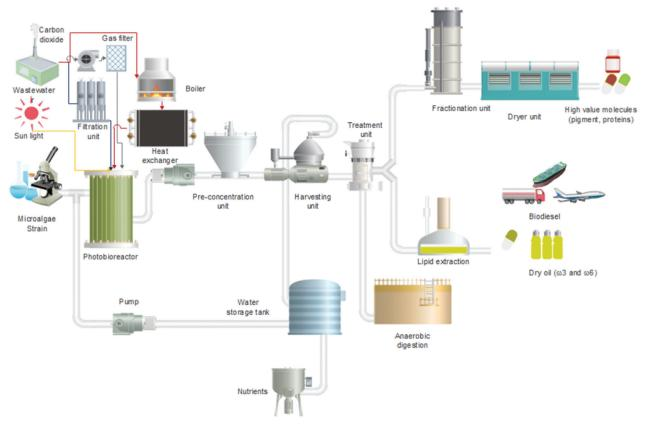
Figure 3. General microalgae production process flow.
