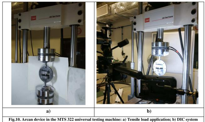
A 3D DIC system was installed to evaluate the displacements and strains of the adhesive interface. During the experimental tests, the corresponding displacement and strain measurements of the adhesive thickness are continuously acquired by processing in-situ images taken by a DIC system from one side. A camera monitors the adhesive layer of the specimen during the loading process.
