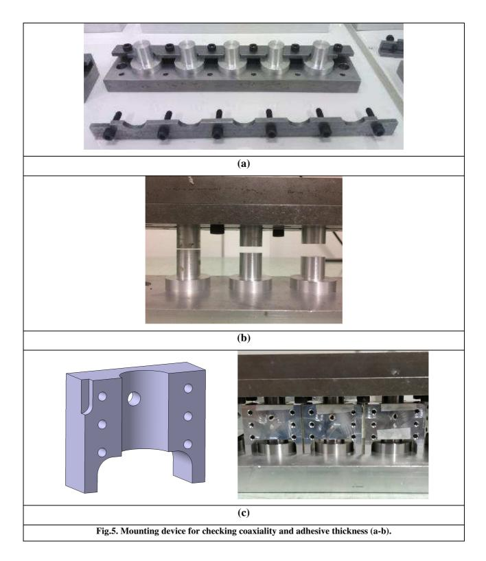
Before bonding, to ensure the bonding effectiveness and to reduce measurement dispersion, the bonding surface quality is controlled by imposing a surface finish as the manufacturing final step. The specified surface roughness  $R_a$  is chosen to be equal to 0.1 µm. The aluminium surfaces are then perfectly cleaned with acetone. In order to achieve co-axiality between the two cylindrical aluminium parts, a mounting system was used as shown in Figure 5 (a) and Figure 5 (b).
