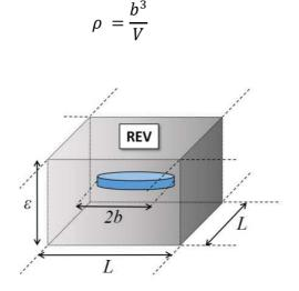
Figure 20: Penny-shape crack (from [35])
