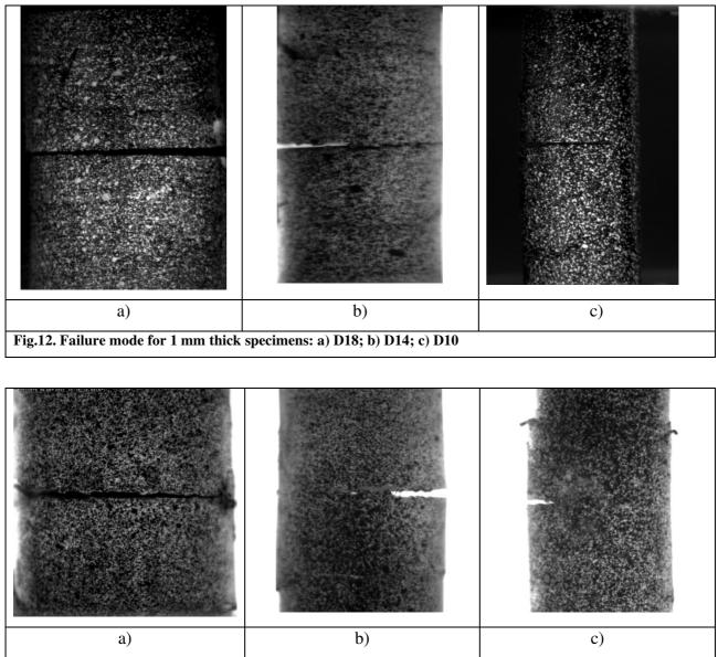
Fig.13. Failure mode for 2.5 mm thick specimens: a) D18; b) D14; c) D10
