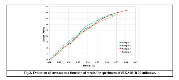
Figure 3 shows the stress-strain curves up to failure. As expected, the adhesives exhibit elastic behaviour, slightly non-linear (due to damage evolution), up to brittle fracture. The Young's modulus, ultimate tensile stress and Poisson's ratio of the SikaDur-30 adhesive are measured and reported in Table 2. These results are close to those quoted by the manufacturer (Table 1).
