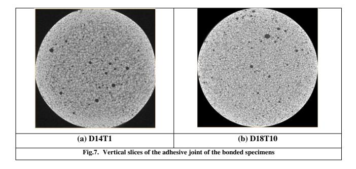
At the end of the reconstruction, each slice of the  $\mu$ Ct scan obtained has the thickness of a voxel (11  $\mu$ m). Sikadur-30 is a filled adhesive, on the slice image the binders can be seen in grey, the colloidal fillers in white and the pores with the lower density appear in black, as shown in Figure 7. In these 3D CT scan images, diffuse porosity is observed for each thickness and diameter of the bond.
