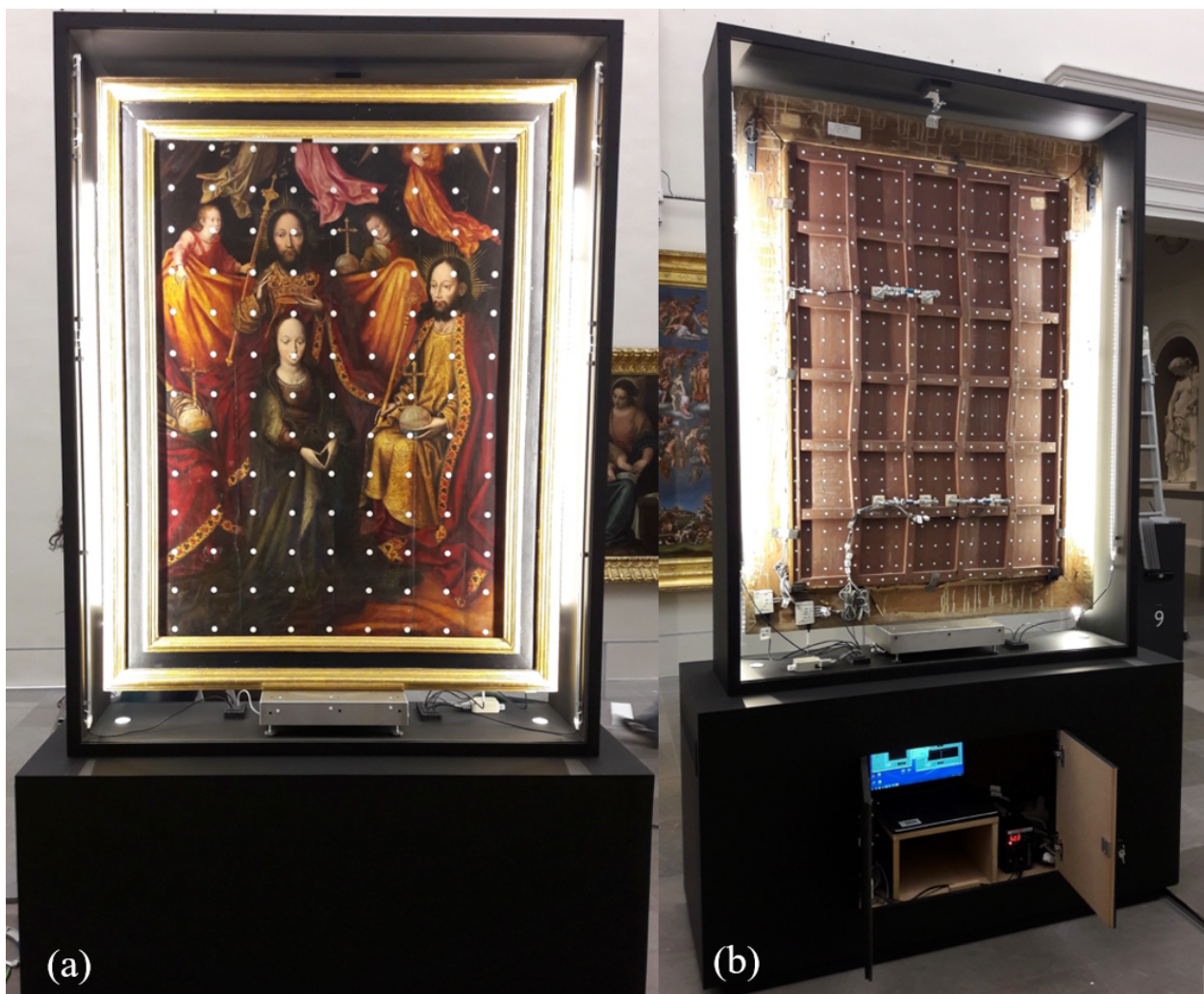
Fig. 1. “ La Sainte Trinité couronnant la Vierge ” with the original frame in the humidity-controlled display case. Markers in the form of round dots positioned on the front (a) and back (b) sides allowed displacement to be measured by stereovision of images, using 4 cameras installed on the walls of the exhibition room.
